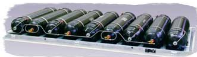
Figure 1-3: Compressed gaseous hydrogen on-board storage (as used in CUTE buses)
