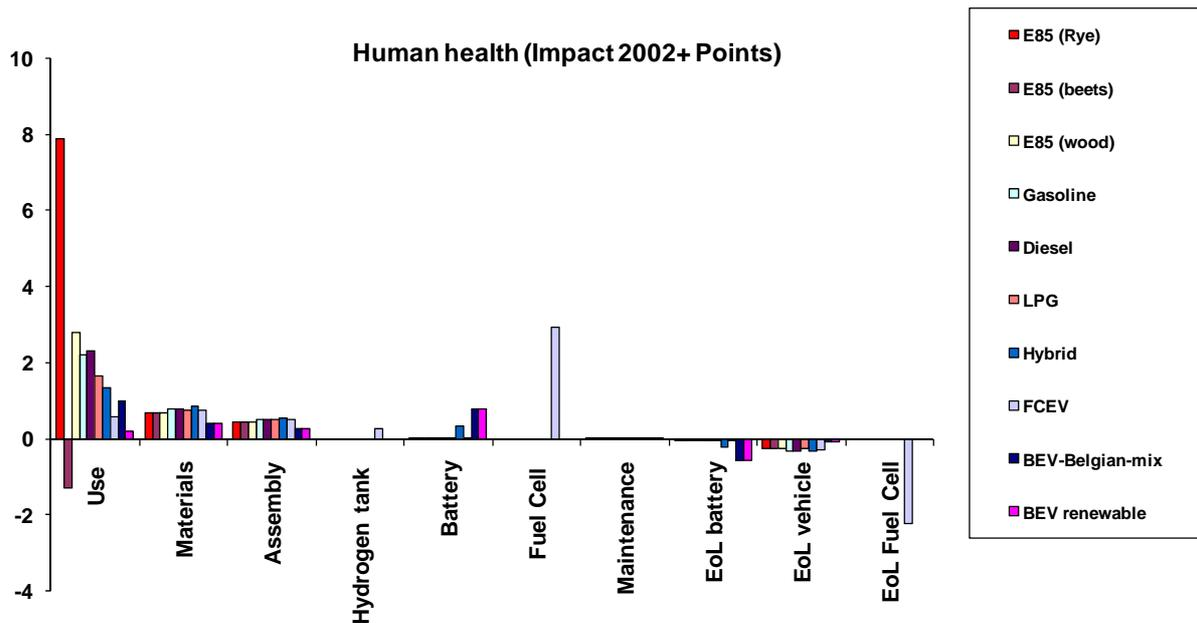
Figure 6: Comparison of the contribution of the different life cycle phases of conventional and alternative vehicles to the impact on human health.
