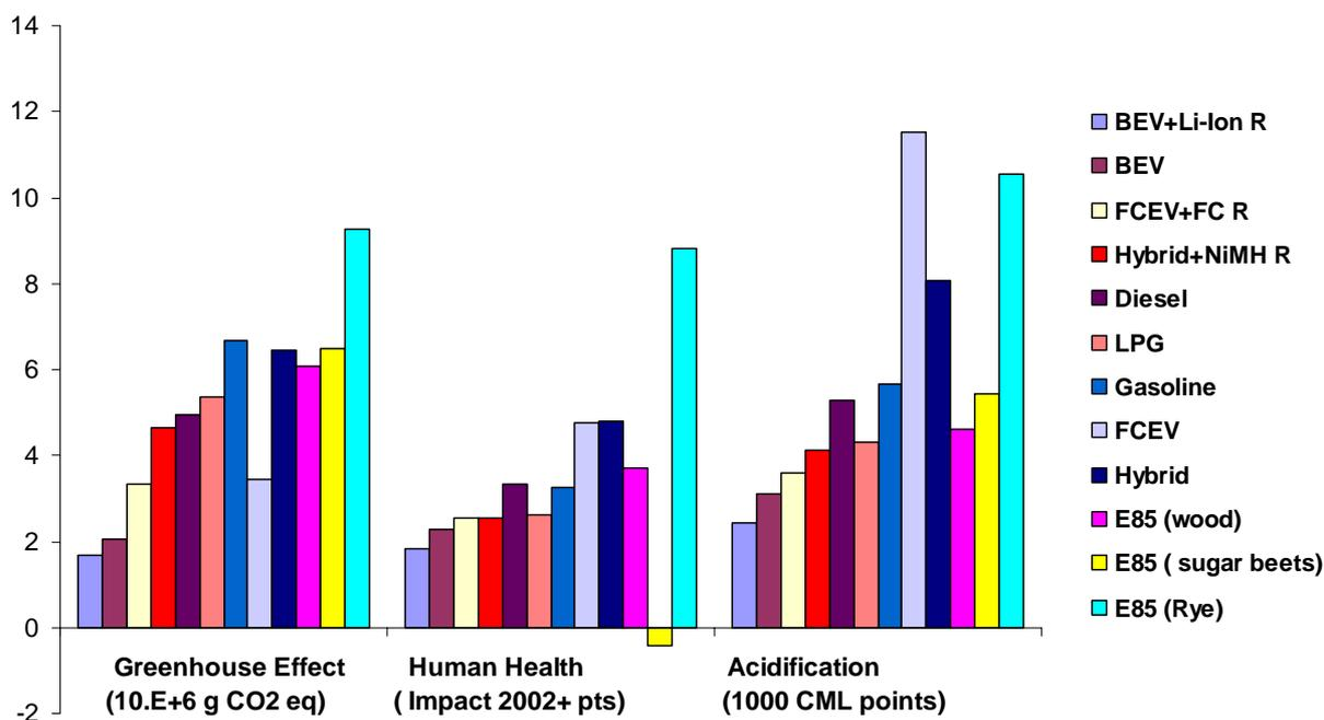
Figure 5: Comparative LCA results of conventional and alternative vehicles from the family car segment (R = Recycling; FC = Fuel Cell).
