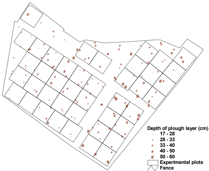
Figure WP2.6: Depth of the plough layer at the Zedelgem site with the location of the experimental plots plotted on top.
