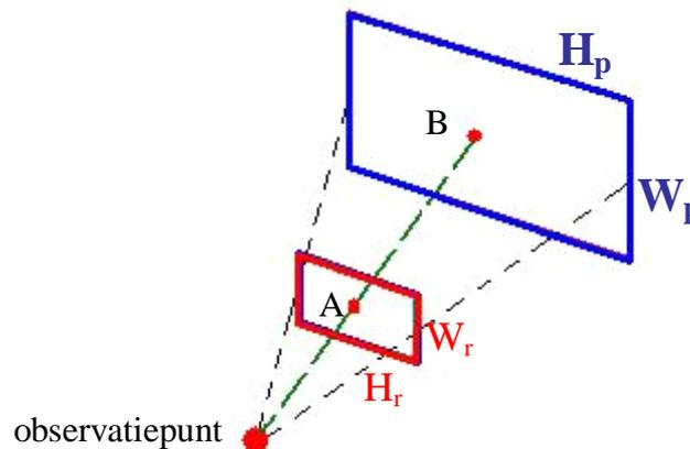
Figure 2-9: Principle of projection of a pixel on a sphere
