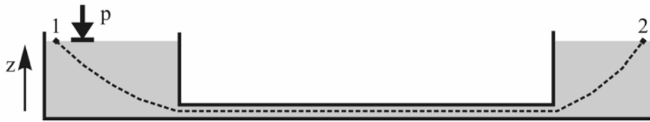
Figure 4-4: Sketch of the stream line in a straight pipeline connecting two reservoirs. The hydrostatic line is considered between two points at equal place height ( z_1 = z_2 ) and with equal minimal velocity ( v_1 = v_2 = 0 ).
