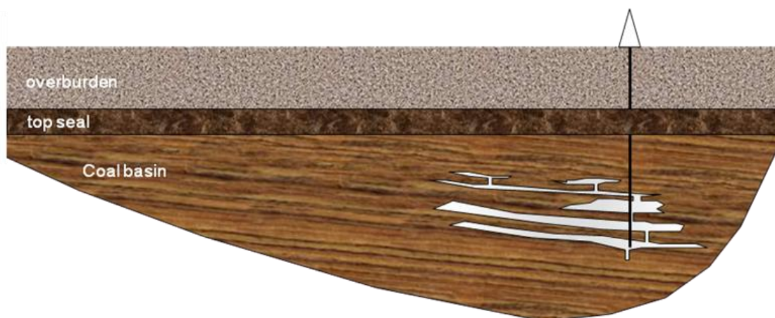
Figure 2.17. Sketch of final CO 2 spread (shown in white) in a hypothetical storage project in the Westphalian coal-bearing sequence of the Campine Basin. Lateral migration is more important than vertical migration and multiple trapping mechanisms are activated (structural, hydromechanical, solution, ionic, mineral, adsorption).
