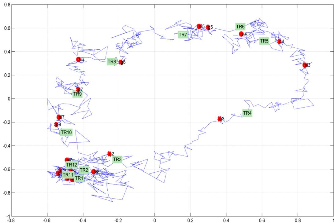
Figure A3-13. Current ellipse reconstructed from all ADCP current measurements (axes are in  $\text{m s}^{-1}$ ). The transect numbers are indicated (TR), as also the positions of vertical profiling on the slope and gully (red bullets: 'g'; 'sl').
