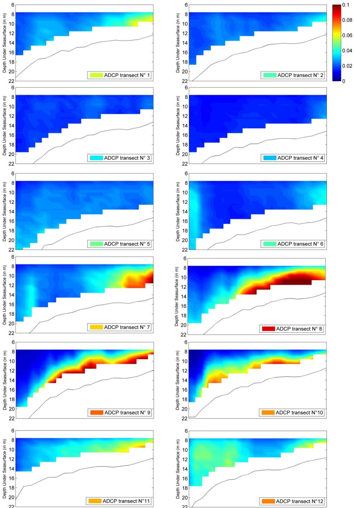
Figure A3-14. Cross-sectional ADCP transects (only downslope) of SPM concentration ( $\text{g l}^{-1}$ ), with reference to the current ellipse of Figure A3-13. The high SPM concentrations in transects 7 to 10 correspond with a turbidity plume, and coincide with the ebbing phase of the tide (NW to SW veering current direction).
