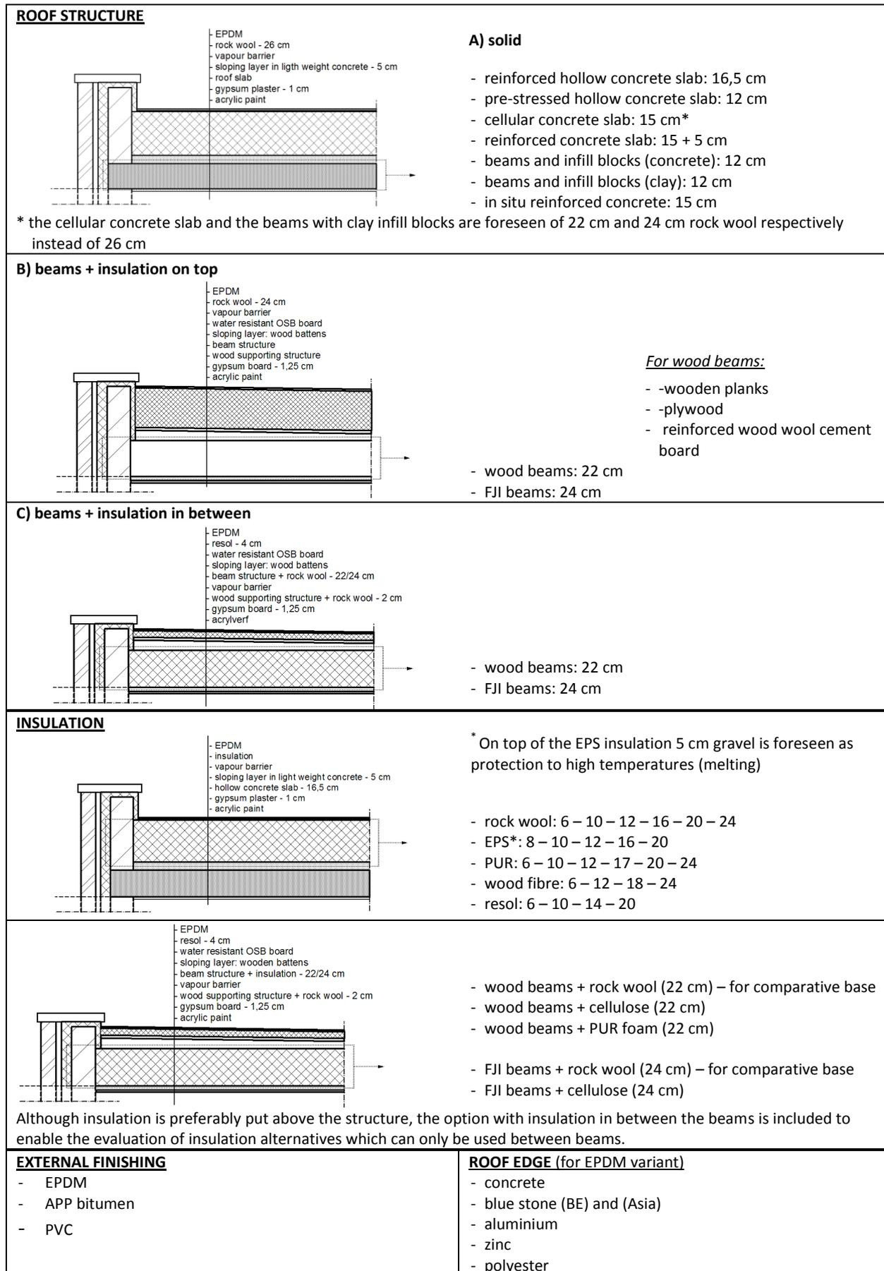
**FIGURE 8** Flat roof: composition of the roof for the optimisation of the different layers
