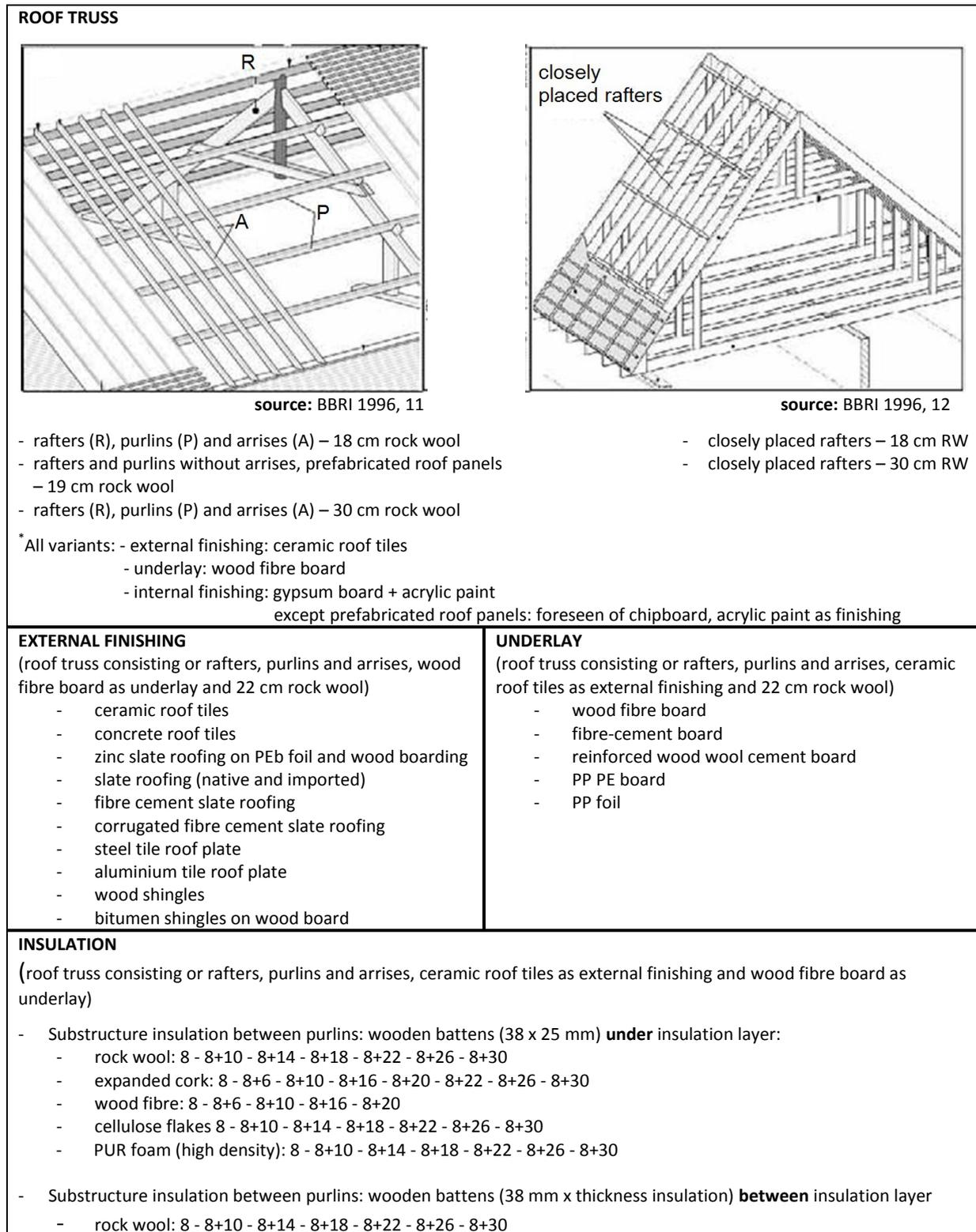
**FIGURE 11** Pitched roof: composition of the roof for the optimisation of the different layers
