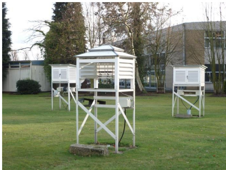
Fig 1: An illustration of a change in the measurement conditions: different types of meteorological shelters (semi-open, closed) have been used since the end of the 19th century in the climatological park in Uccle.
