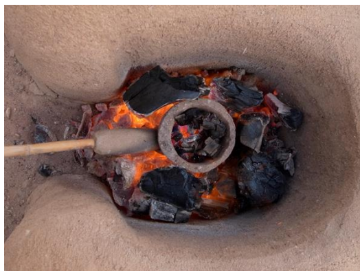
Fig. 2: Copper production. Experimental reconstruction, MRAH - Archéosite d'Aubechies
