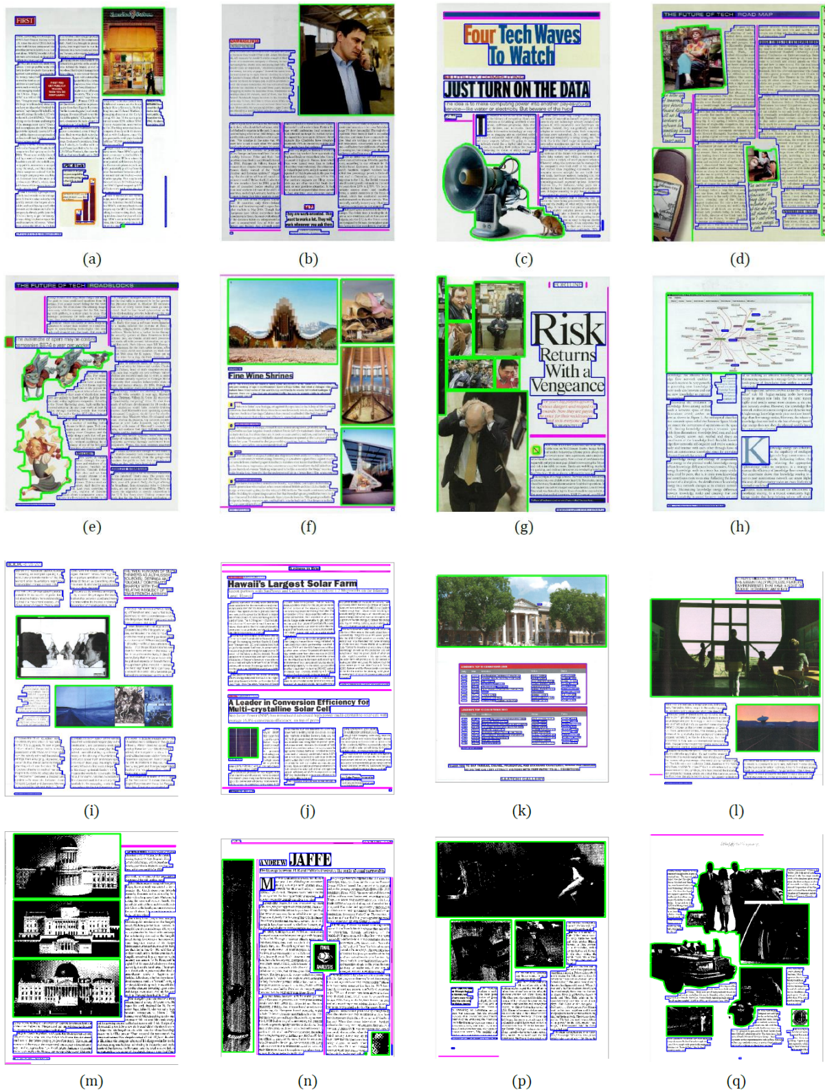
Fig.5 Visualisation of the outputs of DSPH on documents with different style of layouts. Blue, green, blue-violet, orange, magenta represent text, image/graphic, table, chart and separator regions respectively. It can be seen that DSPH operates to derive an accurate parsing of the content of documents with complex layouts.
