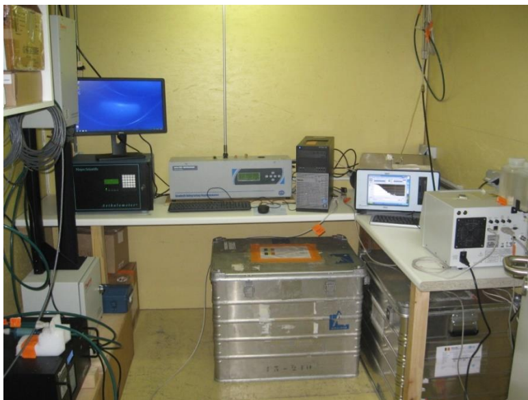
Figure 2: The aerosol in situ instrumentation in the shelter south of the main station; from left to right: TEOM-FDMS, aethalometer, nephelometer, LAS and U-CPC
