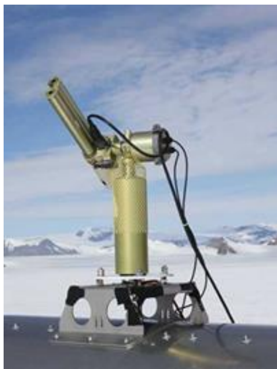
Figure 4: the CIMEL sun-photometer instrument on the Northern roof of the PES.
