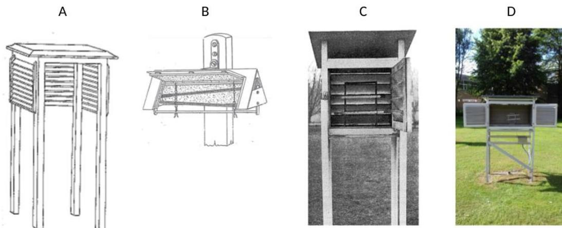
**FIGURE 2:** The different types of exposures and stands used in the network for protecting thermometers. Type A was used from 1880 to about 1910, type B from 1911 to 1920 and type C from 1921 until the 1950s when type D (the Belgian standard of the Stevenson screen) was introduced in the network.
