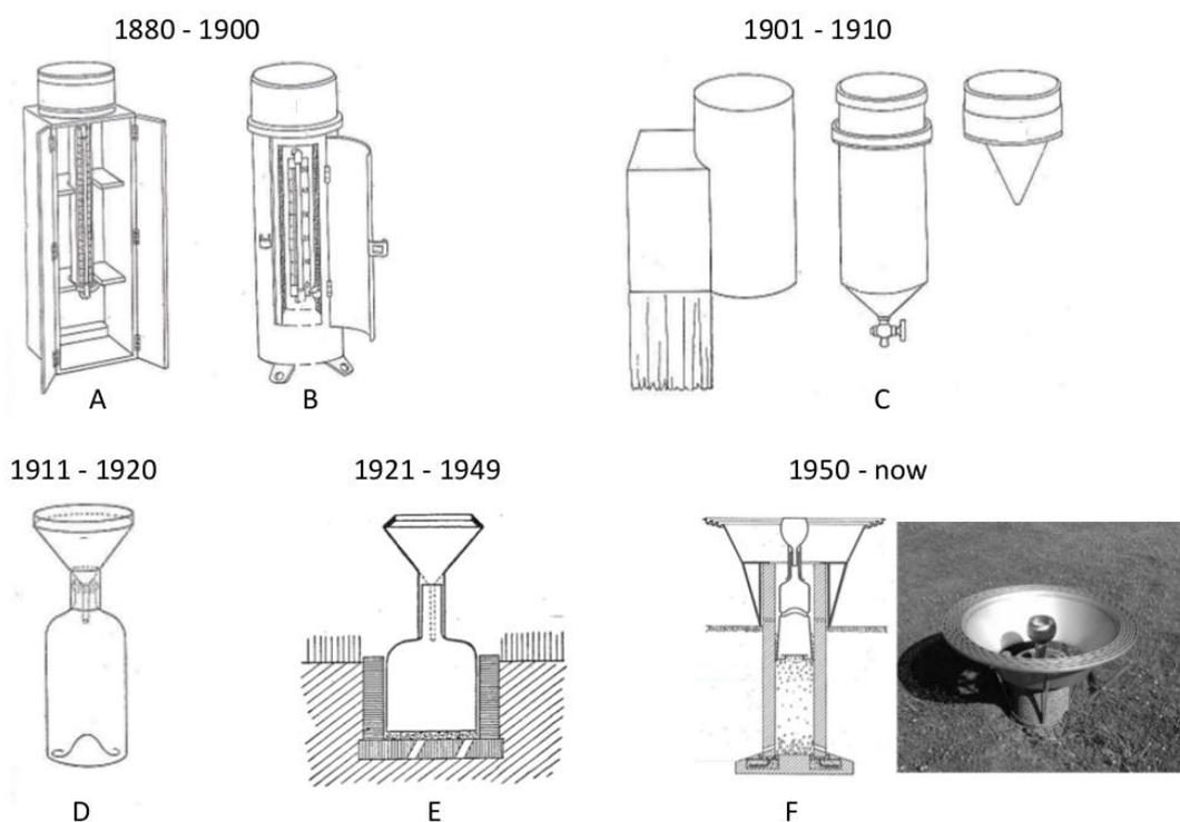
**FIGURE 4:** The different manual rain gauges used in the Belgian climatological network. Note that the indicated time periods are only approximate since the replacement of the instruments was progressive.
