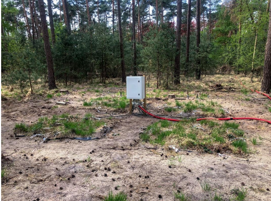
Figure 5: Visualization of a finalized plot. The little layer within the monoliths shows very little destruction while the surrounding of the monoliths suffered a big impact. In the middle of the plot there is the power station for TDRs functioning and data logging.
