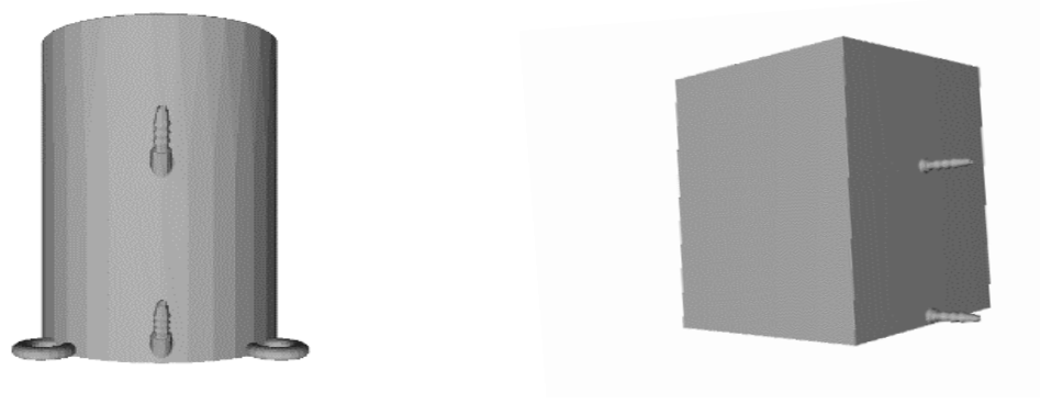
Figure 1: Round and Square samplers for vertical and horizontal installation.
