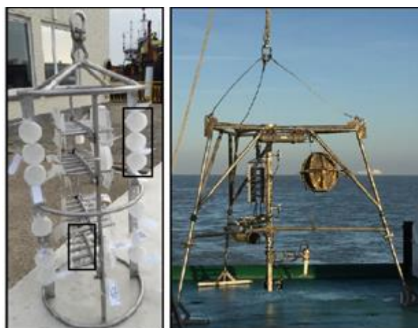
Figure 4. Speedisks and STEPS were mounted on a deployment cage (left) and subsequently attached to a tripod which was lowered onto the seabed at an approximate depth of 10 m (right).
