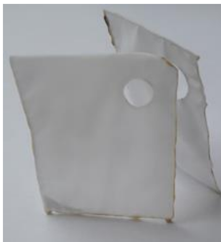
Figure 5. STEPS developed using heat-sealed nylon net filters with dimensions 4x4 cm. The h-DVB sorbent is visible in the lower left corner of the STEPS, yet will be freely dispersed within the nylon mesh when deployed in the water column.
