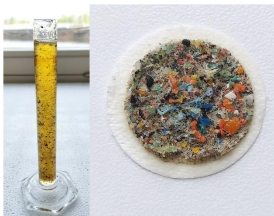
Figure 29. Beach-derived MP mixture (PTX001) suspended in stomach oil of Northern Fulmars and after filtration.
