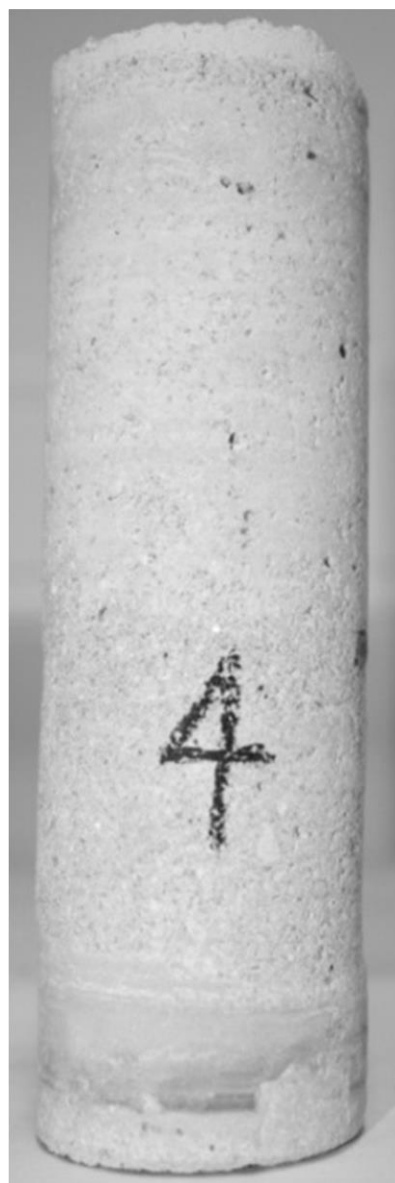
Figure 26: Sample of Pauchot reinforced artificial stone (external wall, Saint-Vincent church)
