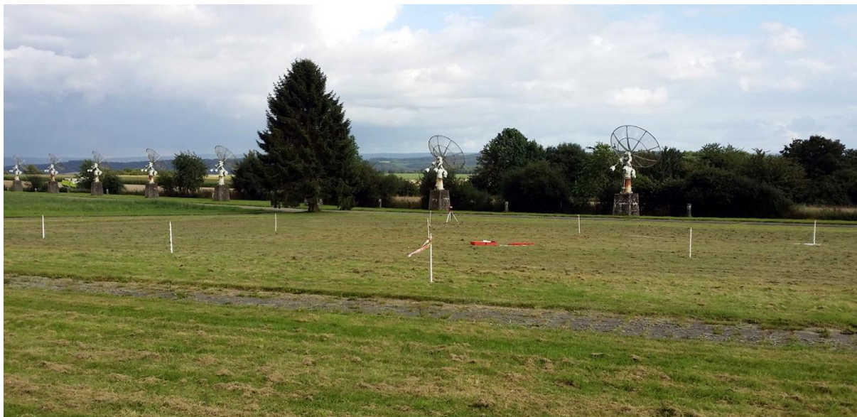
Figure 6 Campaign of on-site measurements of antenna positions (marked by the white sticks)
