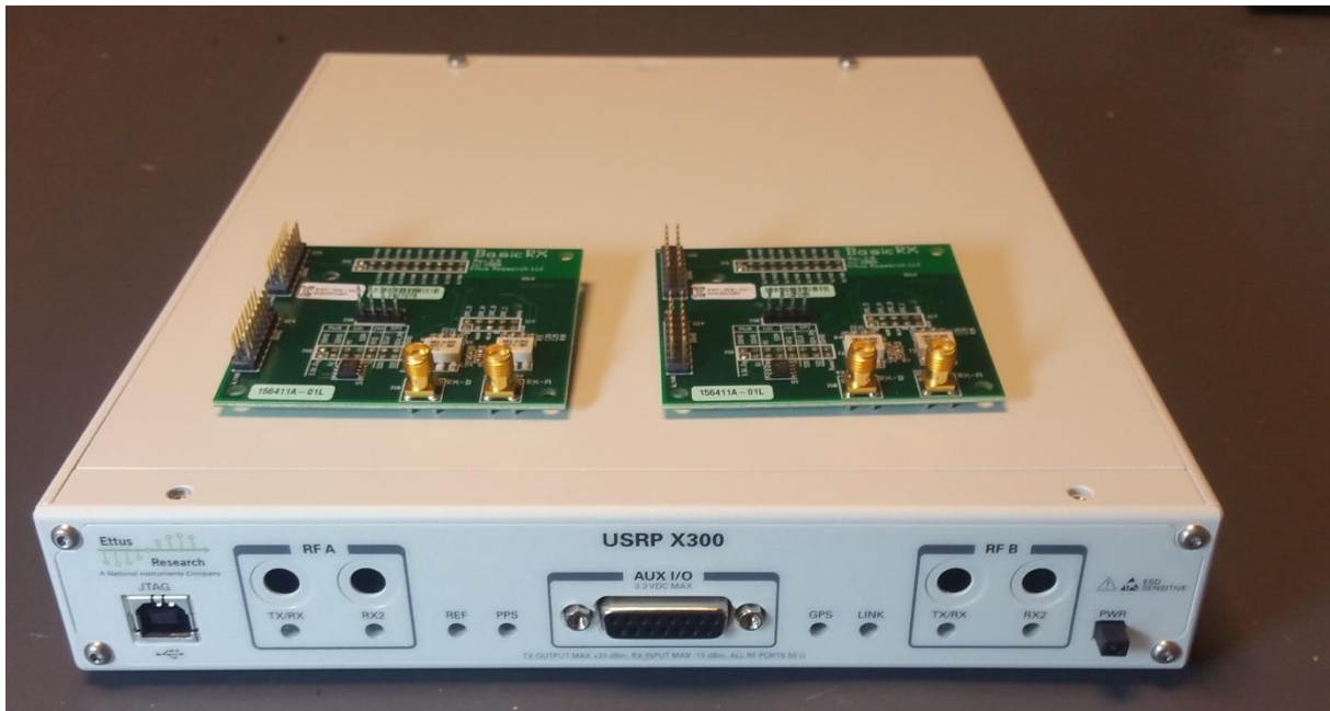
Figure 11 One of the 2 receivers chosen for the project with 2 input cards (each with 2 ports) before integration
