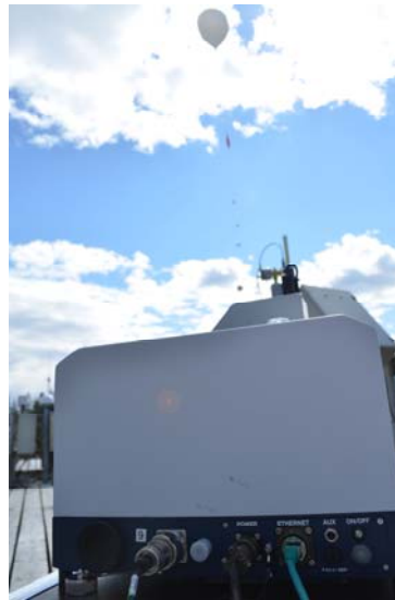
EM27/SUN and aircore launch
