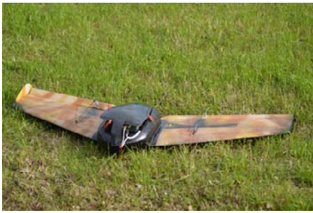
Figure 1: smaller wing 1.4 m wingspan; smaller wing during flight; larger wing 1.75 m wingspan
