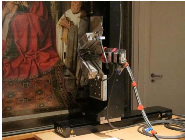
Fig. 5 Prototype of the Macro-XRF scanner developed by Antwerp University (Koen Janssens and Geert van der Snickt)
