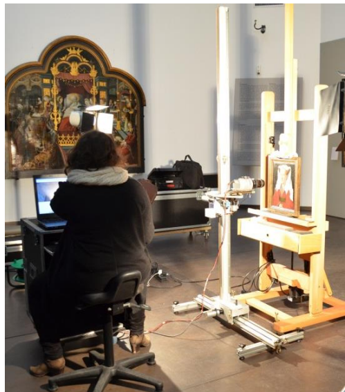
Fig. 4 Mobile rail system developed by Liège University for KIK-IRPA
