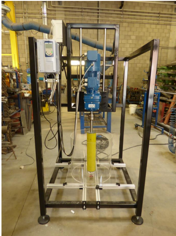
Figure 4.4 - Couette type flocculation reactor, designed and built at KU Leuven, to study sedimentation and aggregation behavior of microplastic (and mineral) particles in an aquatic environment under varying shear flow conditions.
