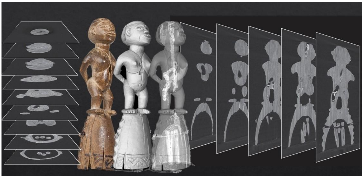
Figure 2: The various ways to visualise the three-dimensional information of a high-resolution scan of a Kongo bell MO.1955.113.17 (10.9 x 3.7 x 2.5 cm, scanned at 62 \mu m) : on both sides of the figure 2D reslices of the bell, in the middle two 3D renderings at different transparency. ©RMCA ©UGCT ©UGent-Woodlab
