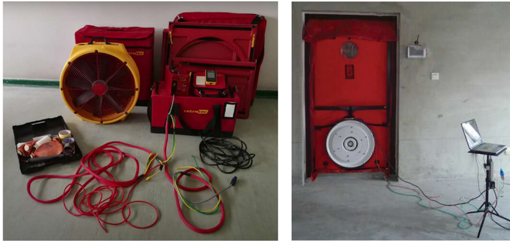
Fig. xxx The blower door equipment (on the left, own studies) and the general configuration of the measurement (on the left, source: Yongming J. and Duanmu L.; https://doi.org/10.1080/23744731.2017.1262707 ).
