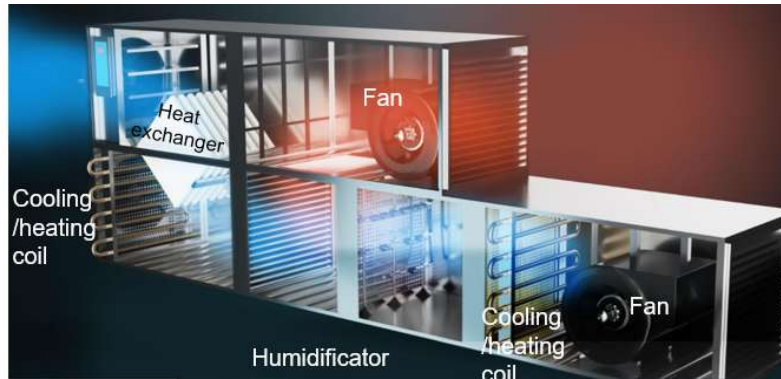
Figure 16: Illustration of an AHU inside and outside ( Source: Airtech Solutions)
