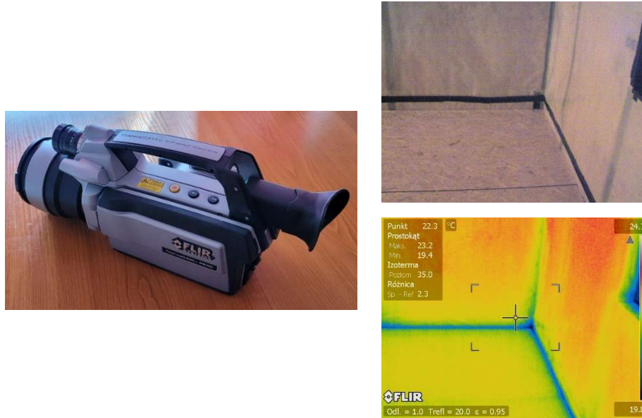
Fig. xxx Infrared thermography: professional infrared camera (on the left), as well as the imaging: digital image (on the top right) and the corresponding infrared image (on the bottom right) (source: own studies).
