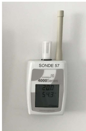
Fig. xxx: T and RH measurements performed on-site: indoors with sonde (on the left) and outdoors with weather station (on the right) (source: own studies).
