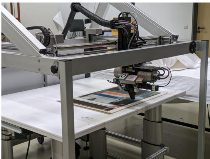
Macro-XRF device scanning an artwork by Léon Spilliaert (photo: Marie-Noëlle Grison)
