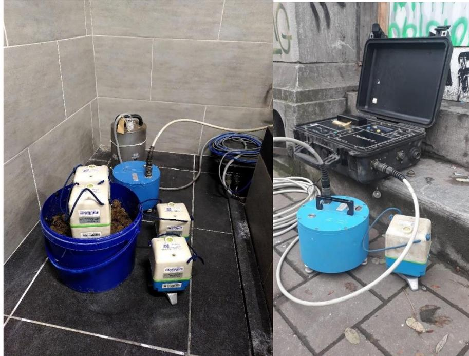
*Figure 5 : Left: Lab-based instrument test of two nodes each based on a tripod or with a spike in a sand-filled bucket next to a classical LE3D/5s (blue pot) seismometer and the well calibrated Guralp sensor of the UCCS permanent station (gray cylinder). Right: Comparison of Lennartz LE3D/5s with city shark digitizer and tripod-based node sensor close the Wiels Cultural Centre in Forest (Brussels).*
