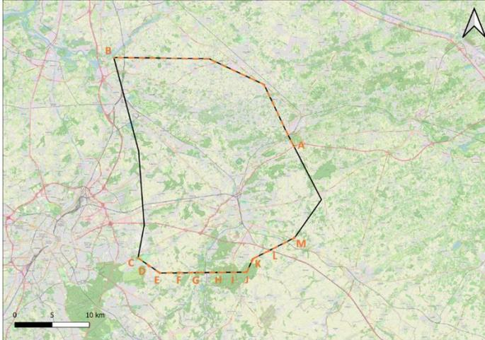
Figure 36. Boundaries conditions prescribed to the seventh layer (Heers Formation) and eighth layer (chalk aquifer) of the numerical model. The orange dotted lines show on which portions the Dirichlet conditions are applied.
