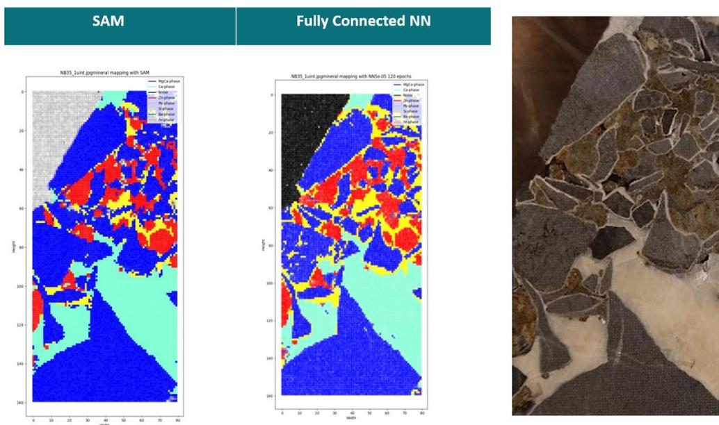
Figure 15: left: example of an automated mineralogical classification made on a Bleiberg Pb-Zn core, comparing the result of the SAM and NN methods, each color represent a specific mineral phase. Right the optical view of the core section, with LIBS ablation points visible.
