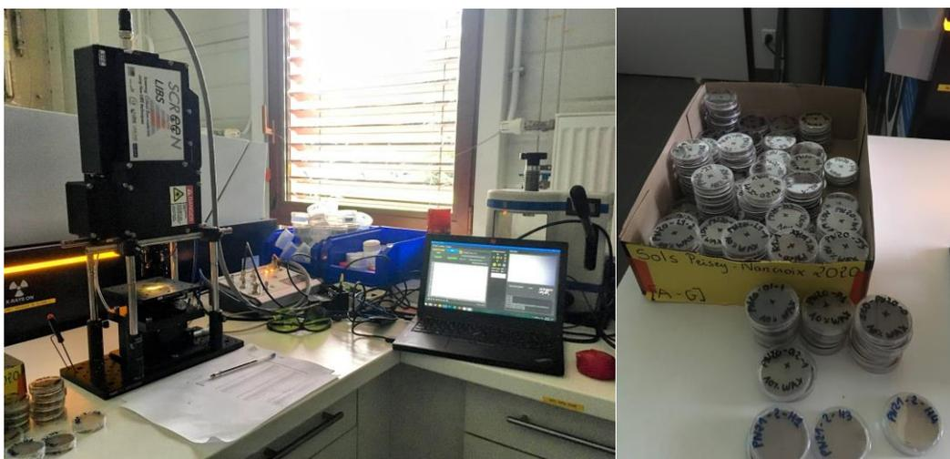
Figure 6: (left) Portable LIBS setup installed at the Edytem laboratory in November 2022 – (right) soil samples dataset.
