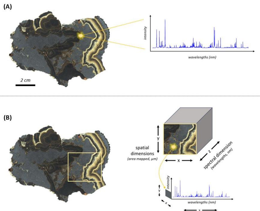
Figure 8. Illustration of LIBS spectra in the difference acquisition methods, A) spot data used in screening and B) data cubes resulting from maps.
