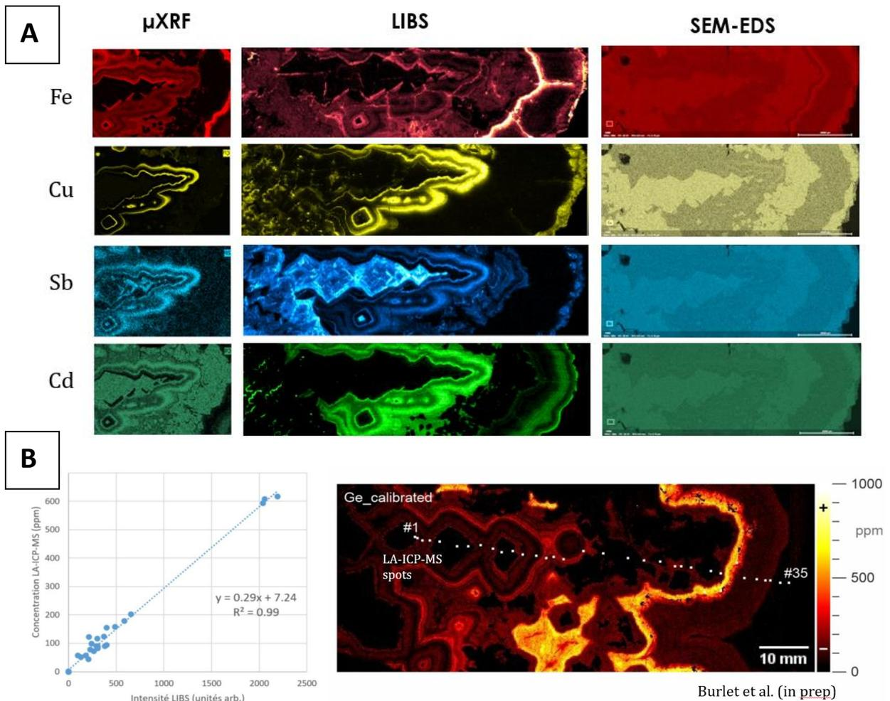
Figure 2: Comparison of selected LIBS maps with different analytical techniques; A) comparison with  $\mu$ XRF and SEM-EDS elemental mapping. B) Comparison with spot analyses of germanium with LA-ICP-MS, where the good correlation allows calibrating the LIBS map based on LA-ICP-MS values.
