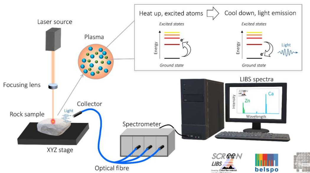
Figure 1: Scheme illustrating the principles of the LIBS technique.
