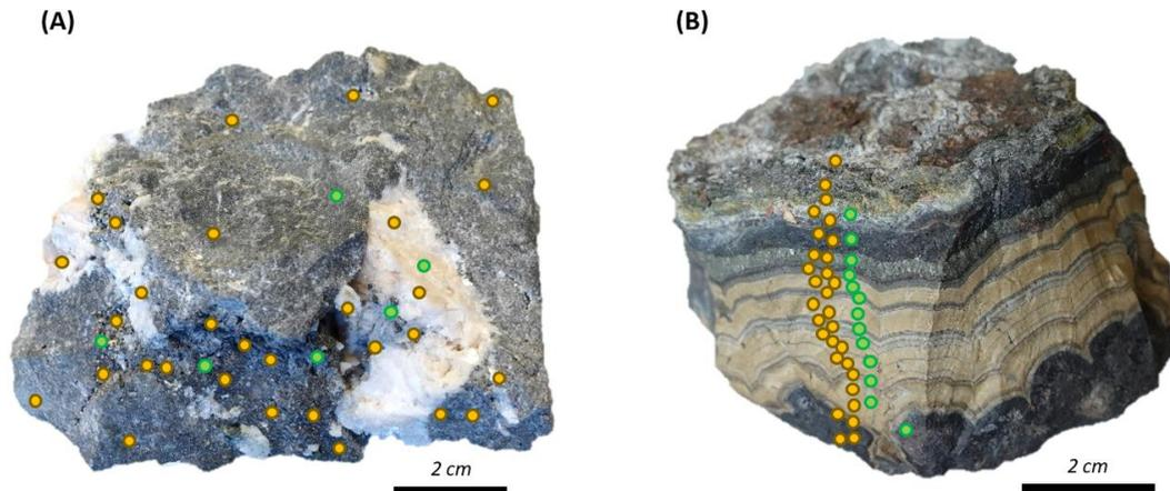
*Figure 4: Schematic illustration of the distribution of LIBS screening spots in hand samples. Green dots represent the targeted screening approach and yellow dots randomised screening – spot size not to scale. (A) Spots in a sample with patchy heterogeneity versus (B) spots in a sample with layered heterogeneity.*
