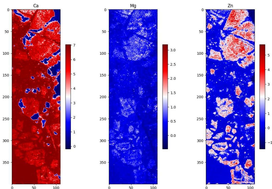
Figure 5: Example of a drill core LIBS image where elemental map have been normalized (SNV method) in preparation for classification
