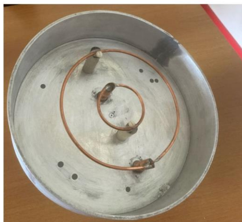
Figure 9: Top Simulation at different frequencies of the chosen feed antenna. Bottom left: feed antenna built by the workshop; bottom right: Beam measured at 1415 MHz
