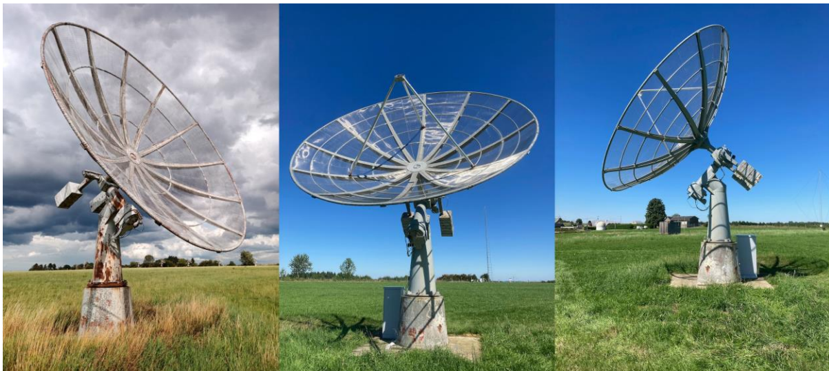
Figure 1: Left initial state of the telescope. Middle and right: view of the telescope after reinstatement, with its new mesh, tripod and control rack
