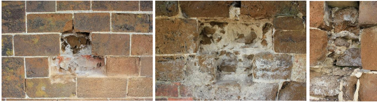
Figure 2: Sampling area of the mortar samples from the south façade at 20.90 m height from the core work (left), the north façade at 11.25 m height, again from the core work at approximately 26 cm depth, (middle) and from the bedding mortar from the north façade at 16.60 m height (right).
