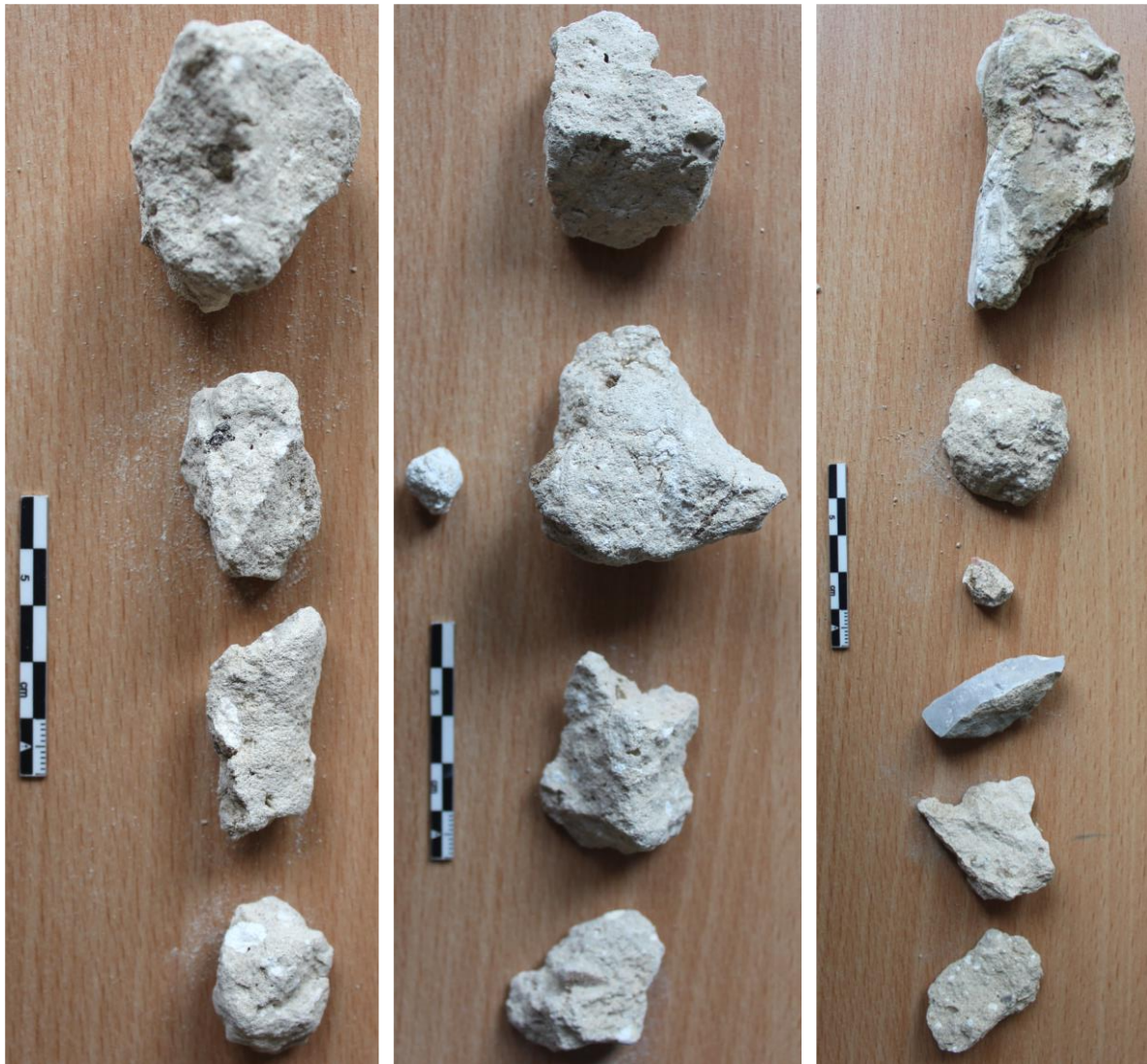
Figure 3: Mortar samples from the south façade at 20.90 m height from the core work (left), the north façade at 11.25 m height, again from the core work at approximately 26 cm depth, (middle) and from the bedding mortar from the north façade at 16.60 m height (right).
