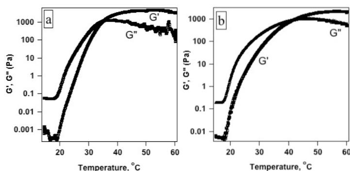
**Figure 6:** Storage moduli ( $G'$ ) and loss moduli ( $G''$ ) for 20% aqueous solutions of di(terpyridine) F127 (a) and di(terpyridine) P105 (b) in presence of 0.5 equivalent Ni(II) as a function of temperature.
