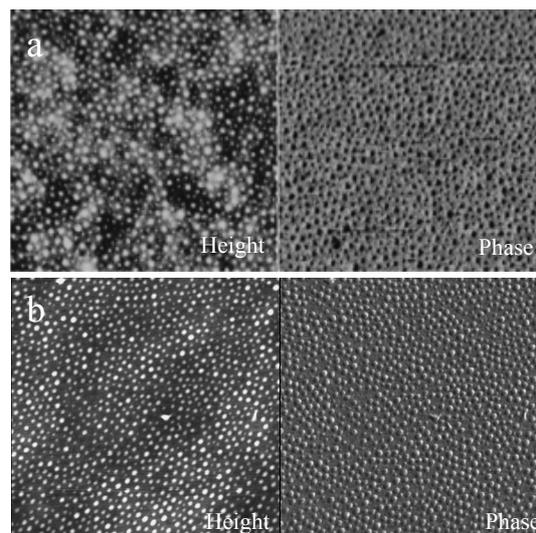
**Figure 2:** AFM images of PS(57500)-P4VP(18500) from 1 wt.% annealed in (a) 1,4-dioxane and (b) chloroform (Scan size: 1.5  $\mu\text{m}$ )
