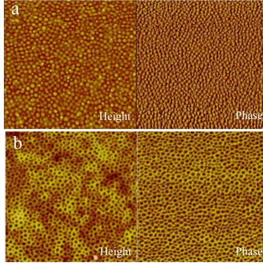
**Figure 6:** AFM images for SMA thinfilm from HNA. (a) before rinsing in methanol (b) after rinsing in methanol (Scan size: 2  $\mu\text{m}$ )
