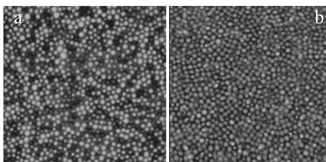
**Figure 4:** AFM height images for SMA thinfilm from HNA annealed in (a) THF (b) 1,4-dioxane (Scan size: 2  $\mu\text{m}$ )
