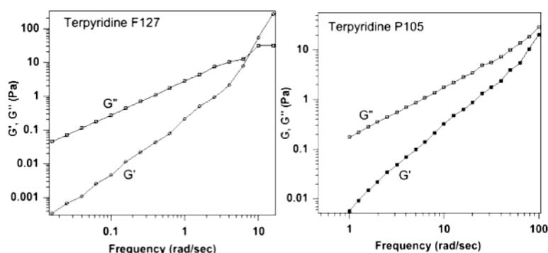
**Figure 5:** Storage moduli ( $G'$ ) and loss moduli ( $G''$ ) for di(terpyridine) Pluronic in presence of 0.5 eq. Ni(II) as a function of applied frequency at 20°C
