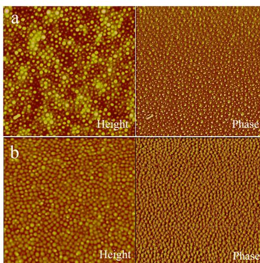
**Figure 3:** AFM images for SMA thinfilm from HNA (a) as spun (b) annealed in 1,4-dioxane (Scan size: 2  $\mu\text{m}$ )
