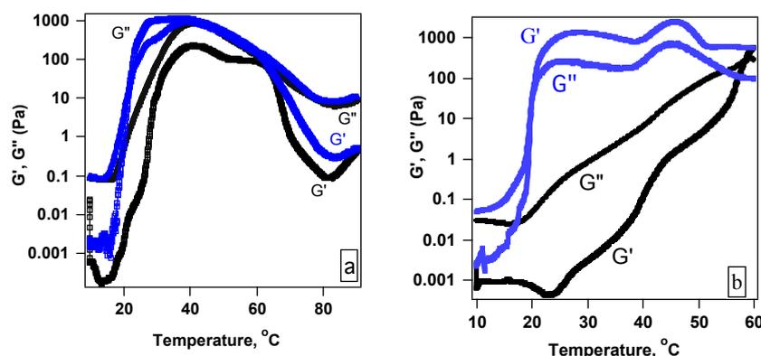
**Figure 9:** Storage moduli ( $G'$ ) for 20% aqueous solutions of di(terpyridine) F127 (a) and di(terpyridine) P105 (b) in presence of 0.5 equivalents of Zn(II) as a function of temperature. heating (black), cooling (blue)
