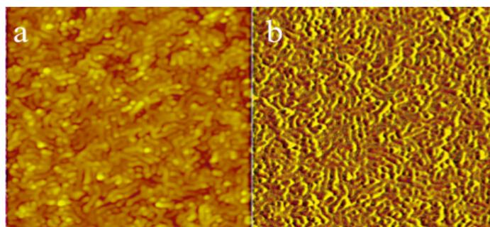
**Figure 5:** *AFM height (left) and phase (right) images for SMA thinfilm from 2wt.% solution in 1,4-dioxane. (Scan size: 3  $\mu$ m)*
