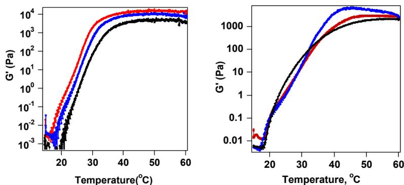
**Figure 8:** Storage moduli ( $G'$ ) for 20% aqueous solutions of di(terpyridine) F127 (left) and di(terpyridine) P105 (right) in presence of different equivalents of Ni(II) as a function of temperature. 0.5 (black), 1.0 (red), 2.0 (blue)
