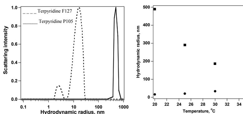
**Figure 1.** (left) CONTIN size distribution histograms obtained for 5 mg.mL<sup>-1</sup> aqueous solutions of Terpyridine Pluronics®, (right) Apparent hydrodynamic radii of 5 mg.mL<sup>-1</sup> aqueous solutions of terpyridine F127 (●) and terpyridine P105 (■) versus temperature.
