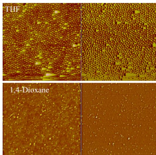
**Figure 8:** The AFM images for the thin films of 1 wt.% SMA solution of PS(57500) - P4VP(18500) mixed with equimolar amount of ADCA from THF and 1,4-dioxane solutions
