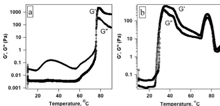
**Figure 3:**  $G'$  (storage moduli) and  $G''$  (loss moduli) for 20% di(terpyridine) F127 (a) and di(terpyridine) P105 (b) as a function of temperature.
