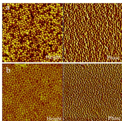
**Figure 7:** The AFM images for the thin films of 1 wt.% pure PS(22000)-P4VP(22000) (a) and mixed with HNA(b) in 1,4-dioxane solutions
