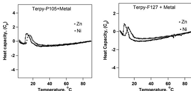
**Figure-11** Modulated DSC thermograms for aqueous solutions of terpy-Pluronics in presence of transition metal ion.
