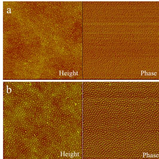
**Figure 1:** AFM images of PS-P4VP thin film spin-coated on silicon substrate from 1 wt. % (a) and 2 wt.% (b) concentration in 1,4-dioxane (Scan size: 2  $\mu\text{m}$ )
