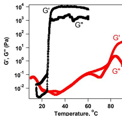
**Figure 4:** Changes in the storage moduli ( $G'$ ) and  $G''$  (loss moduli) as a function of temperature for 20% aqueous solutions of F127 (black) and P105 (red) in presence of 0.5 equivalent Ni(II).
