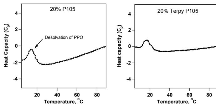
**Figure-10** Modulated DSC thermograms showing complex heat capacity.
