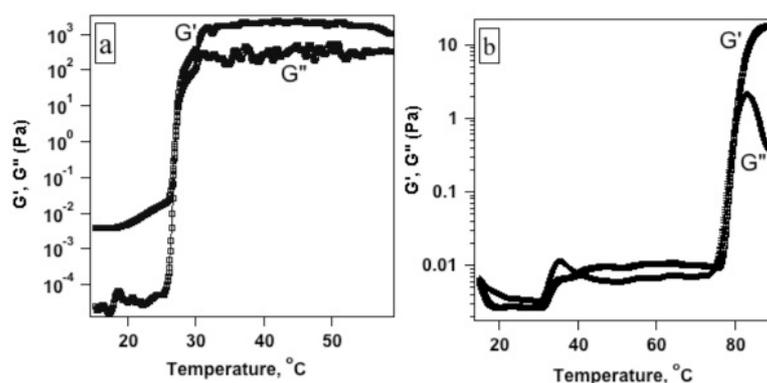
**Figure 2:**  $G'$  (storage moduli) and  $G''$  (loss moduli) for 20% F127 (a) and 20% P105 (b) as a function of temperature.
