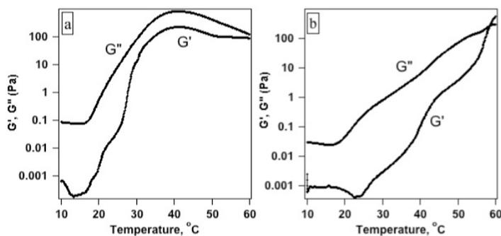
**Figure 7:** Storage moduli ( $G'$ ) and loss moduli ( $G''$ ) for 20% aqueous solutions of di(terpyridine) F127 (a) and di(terpyridine) P105 (b) in presence of 0.5 equivalent Zn(II) as a function of temperature.
