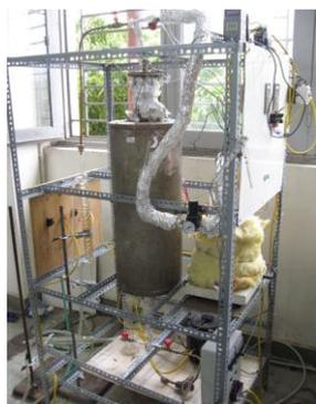
**Fig. 53,** Microreactor for the concentration of ethanol by adsorption on zeolite adsorbent
