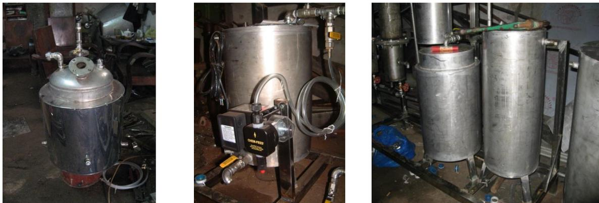
**Figure 55**, Evaporator (left), ethanol pump (center) and ethanol fuel stock tank (right) with liquid-vapor separator
