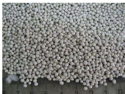
**Figure 58**, Photograph of Zeolite A adsorbent
