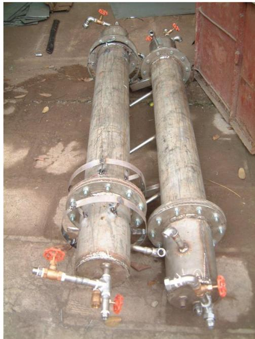
**Figure 59**, Adsorption columns
