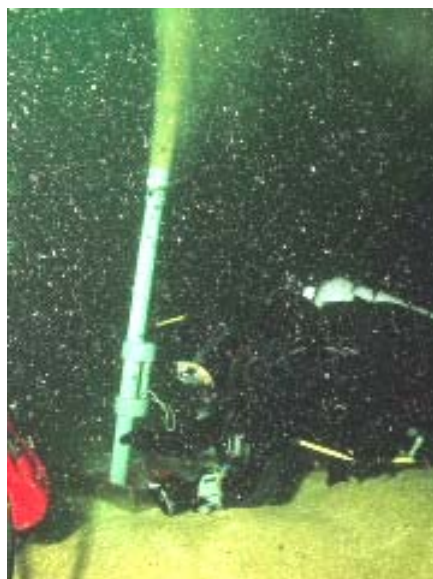
Photo 1 Soft sediment sampling using air-lift. Kilmore wreck 2005
