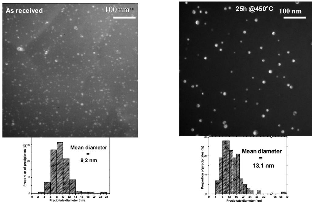
**Figure A.5.3:** Comparison of the size of nano-sized  $\text{Al}_3(\text{Sc}_x\text{Zr}_{1-x})$  precipitates in the AR material and after 25h at 450°C
