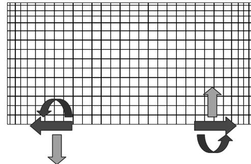
**Figure E.5.3: Meshing and boundary conditions**
