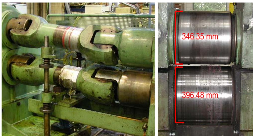
**Figure 1.4: Line-up for the twin drive, different diameters**
