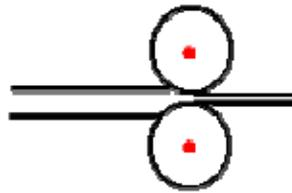
**Figure 1.1: Performed conventional cold rolling (roll diameter 396 mm)**
