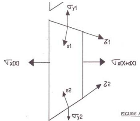
**Figure A.12.2: Static equilibrium of a slice in the rolling direction**
