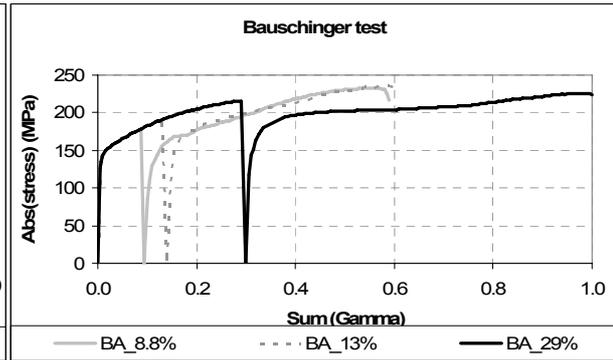
**Figure A.1.8: Experimental Bauschinger tests (8.8, 13 and 29%)**
