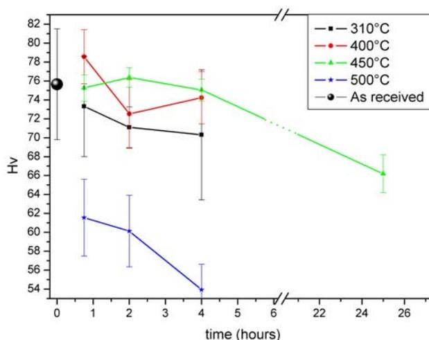
**Figure A.5.1: Hardness evolution versus the duration of heat treatment realized at different temperatures.**
