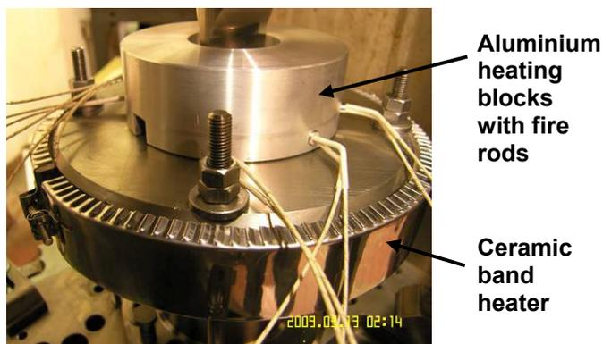
**Figure 2.5: Heating elements for I-ECAP of bars**
