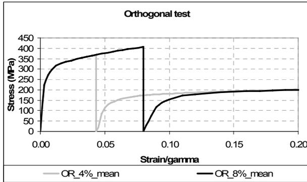
**Figure A.1.7: Experimental orthogonal tests (4 and 8%)**
