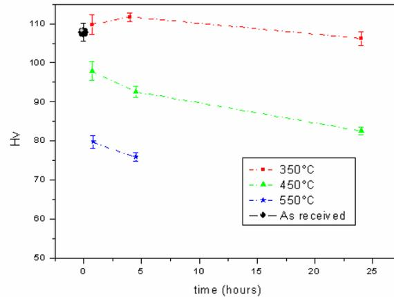
**Figure A.9.1: Thermal stability of the AR 7.2 mm thick plate**
