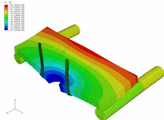
**Figure 2.11: Deflection of screw jack supporting plate**
