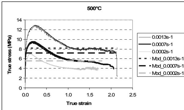
**Figure A.1.12: Superplasticity tests at 500°C**
