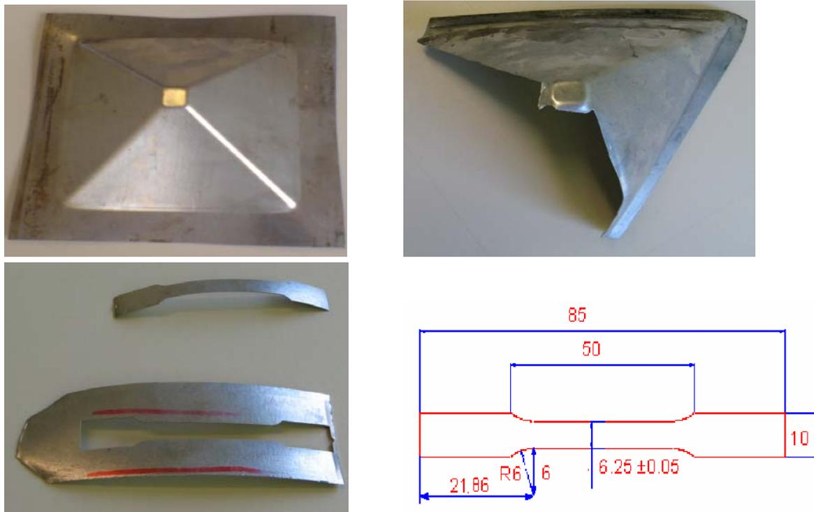
**Figure A.3.3: Tensile test specimen**
