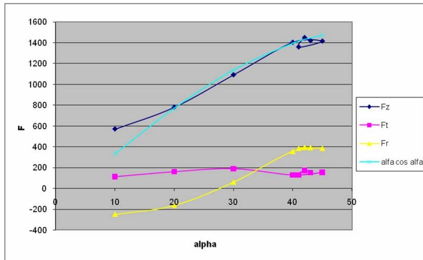
**Figure C.3.1: AA2024: Force components for different wall angle**
