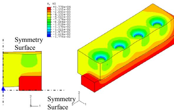
**Figure 2.10: Deflection of die due to bolt tightening**
