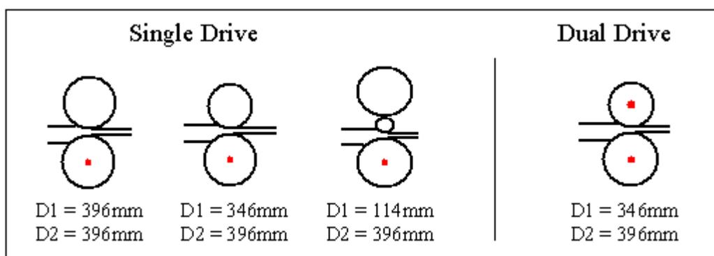
**Figure 1.2: Performed asymmetrical cold rolling configurations**
