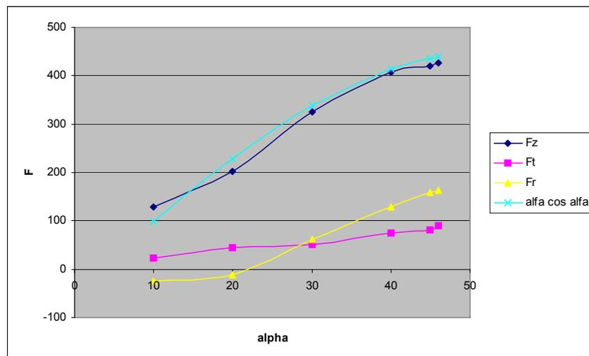
**Figure C.3.2: AlMgSc: Force components for different wall angle**
