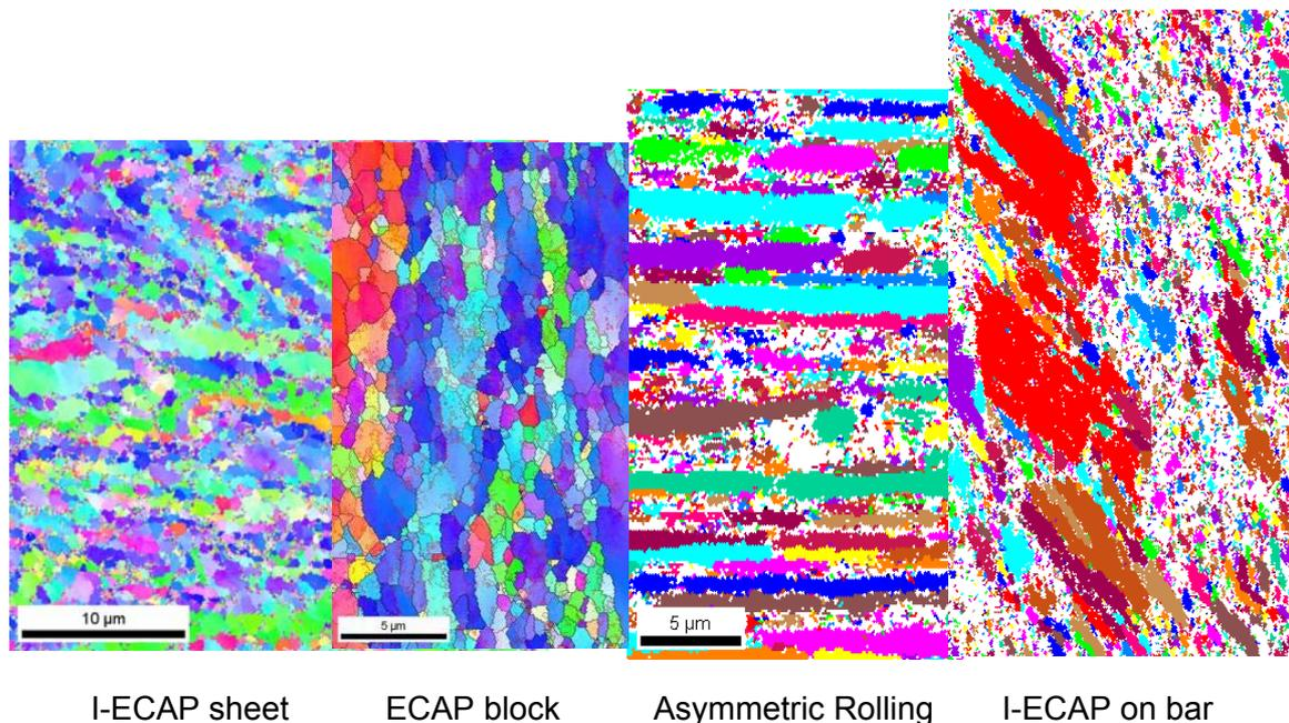
**Figure B.1.1: Overview of the microstructure obtained after various methods of severe plastic deformation, applied on a Al-Mg-Sc alloy**
