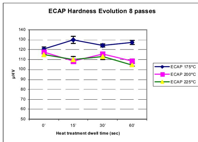
**Figure A.8.2: Thermal stability of samples ECAP'ed at 175°C, 200°C and 225 °C and annealed at the same temperature**
