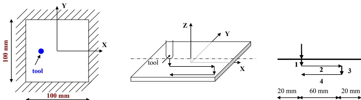
**Figure A.2.13: Description of the Line test: geometry and tool displacements**
