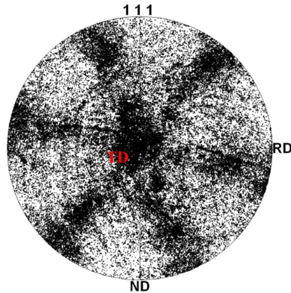
**Figure A.4.5: 111 pole figure of an I-ECAP sheet**
