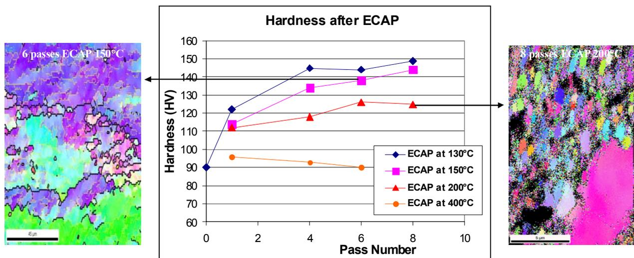
**Figure A.8.1: Hardness of cylindrical ECAP samples after various ECAP passes at different temperatures. Substructure after 6 passes at 150°C (left) and 8 passes at 200°C (right)**
