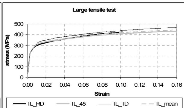
**Figure A.1.5:** Experimental shear tests and average curve **Figure A.1.6:** Experimental large tensile tests and average curve
