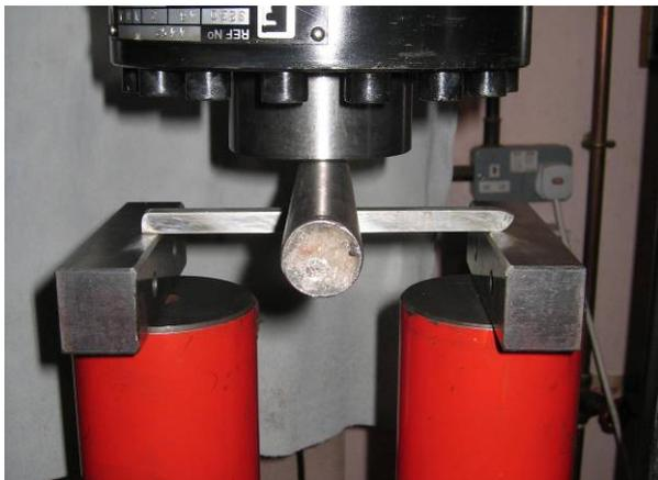
**Figure 2.14: Straightening of bars using 3- point bending**
