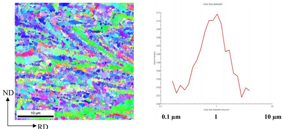
**Figure A.4.4: (a) EBSD scan on a longitudinal section of an I-ECAP'ed sheet and (b) grain size distribution**
