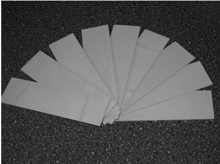
**Figure A.4.1: Conversion coated strips**
