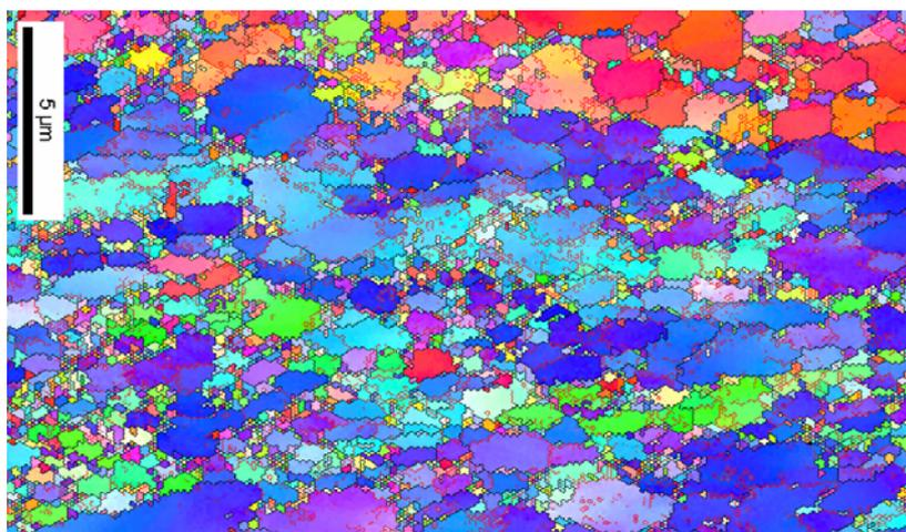
**Figure A.10.1: Transverse section of a rectangular ECAP sample after 8 passes at 200°C (route C)**
