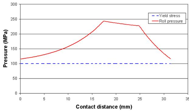
**Figure A.12.3: Pressure distribution along the contact length**
