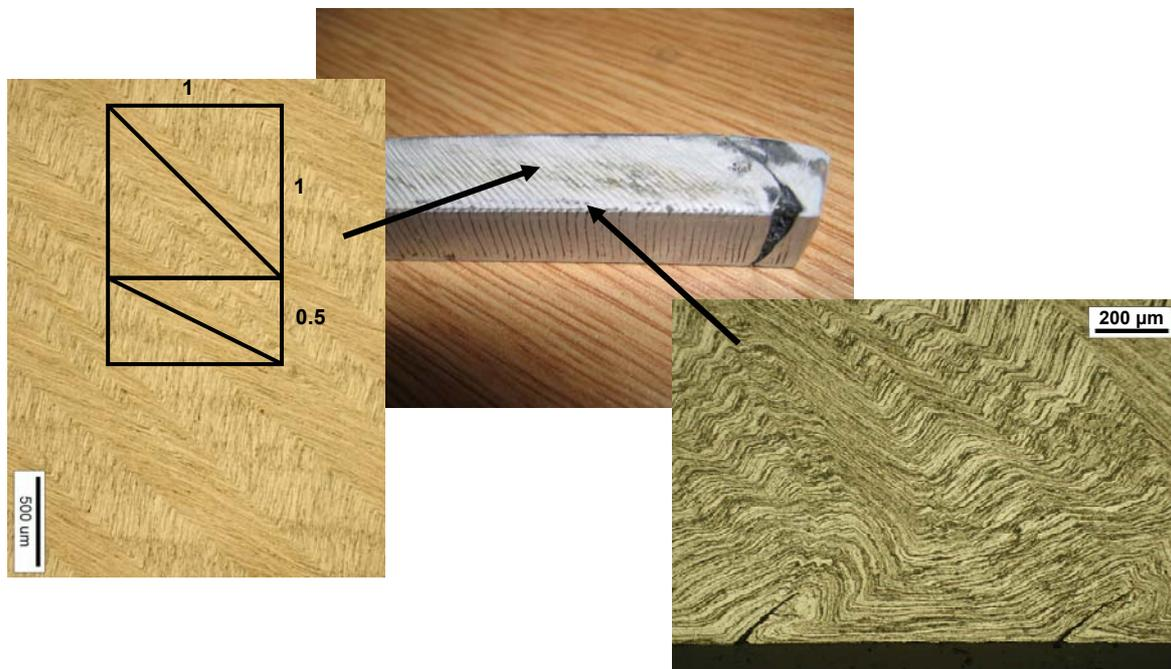
**Figure A.6.1: Shear band strain localisation during 2<sup>nd</sup> pass of I-ECAP at room temperature**
