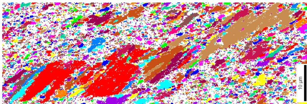
**Figure A.6.5: (Partial) EBSD scan of the longitudinal section of a sample after 6 I-ECAP passes**
