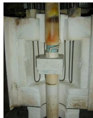
**Fig. 3.5: Uniaxial hot pressing setup**
