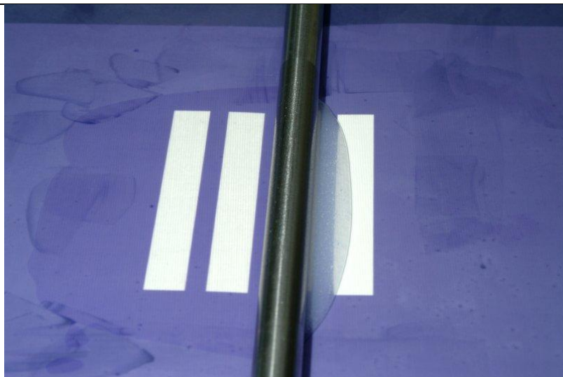
Fig. 26: Illustration of screen printing method used. The basic screen mask consists of 4 rectangular shapes (8x1 cm); the picture show the bar as it is moving over the screen. The silicone is also visible.
