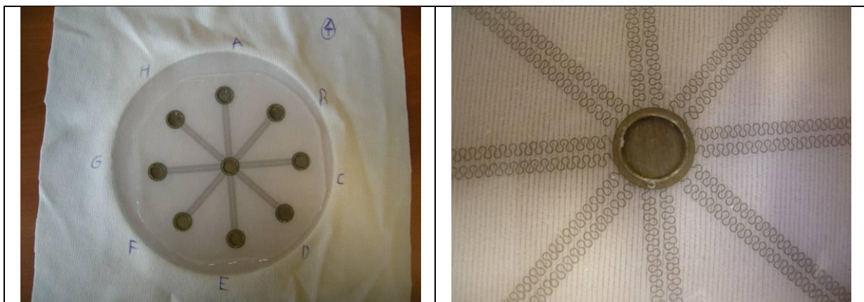
Fig. 34: Electronic interconnection structures, integrated on textile
