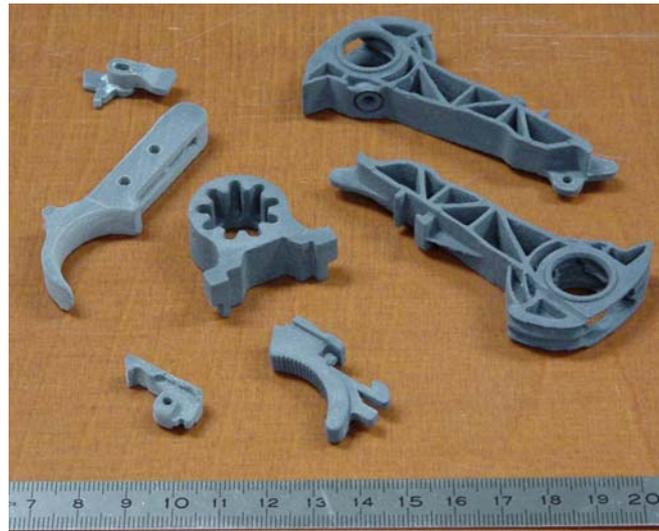
**Figure 12: complex parts in SiC (green parts)**
