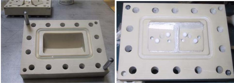
**Figure 24: RTM mould**
