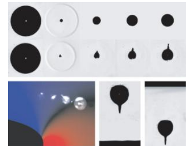
Cavitated bubble collapse on parabolic flights (EPFL)
