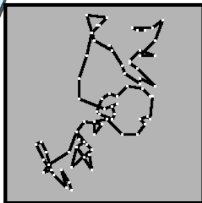
Brownian motion of a particle during free-fall in the drop-tower (Univ Braunschweig)
