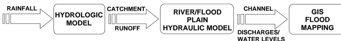
Figure 36. Schematic representation of river flood modeling.
