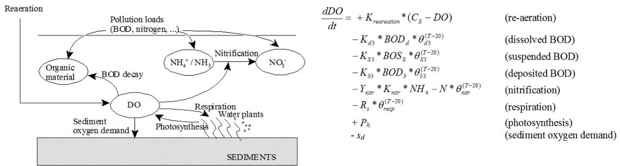
Figure 55. Overview of physico-chemical water quality processes considered in the model for the oxygen cycle.
