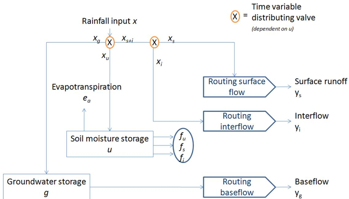
Figure 38. Generalized lumped conceptual rainfall-runoff model structure, considered by the VHM approach.
