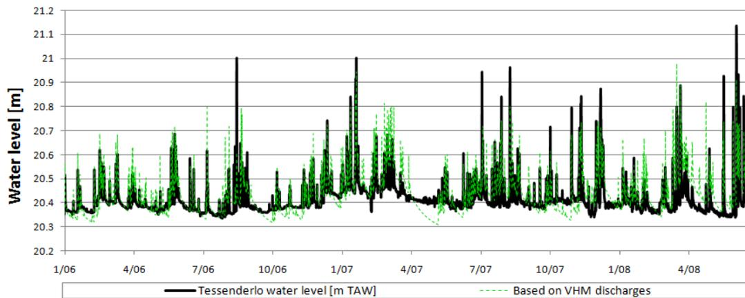
Figure 49. Comparison of hourly observed water level series at Tessenderlo station with the MIKE11 model results after simulation of VHM rainfall-runoff input.
