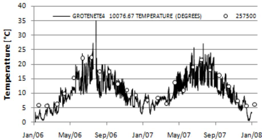
Figure 61. Comparison of observed and modeled water temperature values at Varendonk station.
