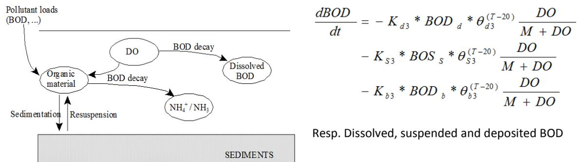
Figure 56. Overview of physico-chemical water quality processes considered in the model for the organic pollution cycle.
