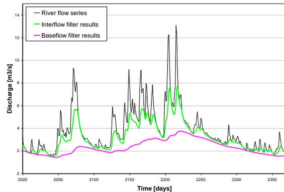
Figure 40. Baseflow and interflow filter results for the observed series at Varendonk station.
