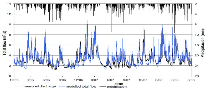
Figure 44. Comparison of hourly observed river flow series at Varendonk station with the VHM model results.
