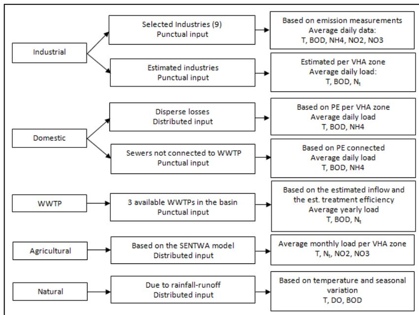
Figure 59. Summary of the pollutant sources introduced in the water quality model of the Grote Nete basin.
