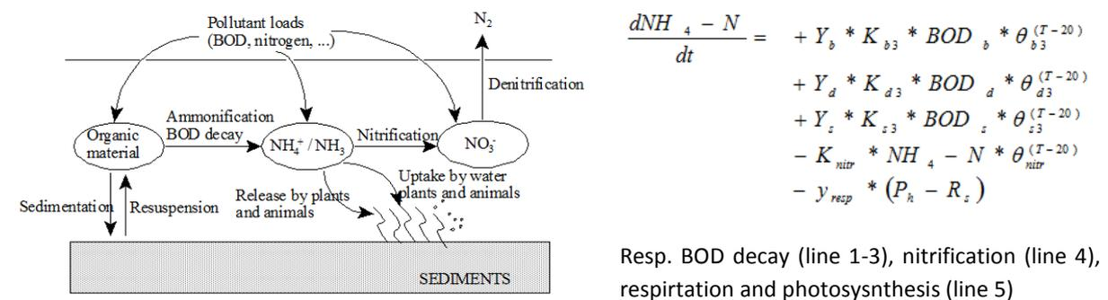
Figure 57. Overview of physico-chemical water quality processes considered in the model for the nitrogen cycle
