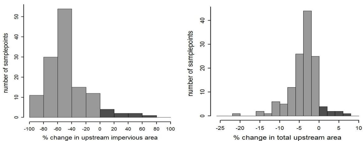
Figure 70 a and b: For the different points (n=131) the difference in upstream impervious areas was calculated between natural upstream areas and upstream areas with the WWTPs connected areas included. Upstream impervious area could decrease by 99% or increase by 64%. Total upstream areas changed between -16% and 3%.
