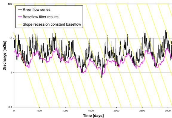
Figure 39. Baseflow filter results for the observed series at Varendonk station.
