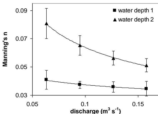
The flow resistance also depends on the water depth. For an identical biomass, the friction increases for a lower water depth (Figure 67). This is evident as the biomass is compacted to a smaller volume. The flow resistance decreases with higher flow, but this is more outspoken for higher water levels. In reality, there is a complex relation between flow resistance, hydraulic head (water) level, flow velocity and flow volume. But these relations are dependent on species composition.
