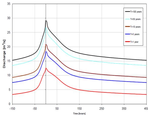
Figure 53. Composite hydrographs for 1, 5, 10, 50 and 100 years for the Grote Nete River at Varendonk station.
