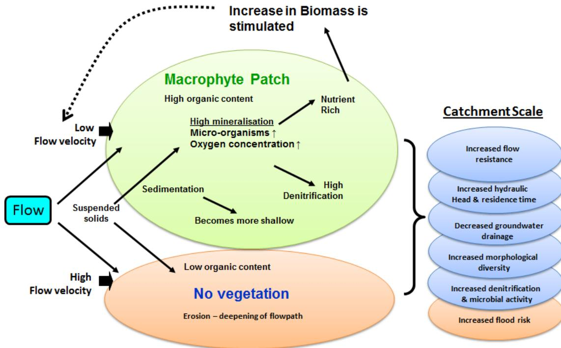
Figure 63: Feedback mechanisms between hydraulics, flow velocity, vegetation composition, nutrient availability, physical stress, and more....
