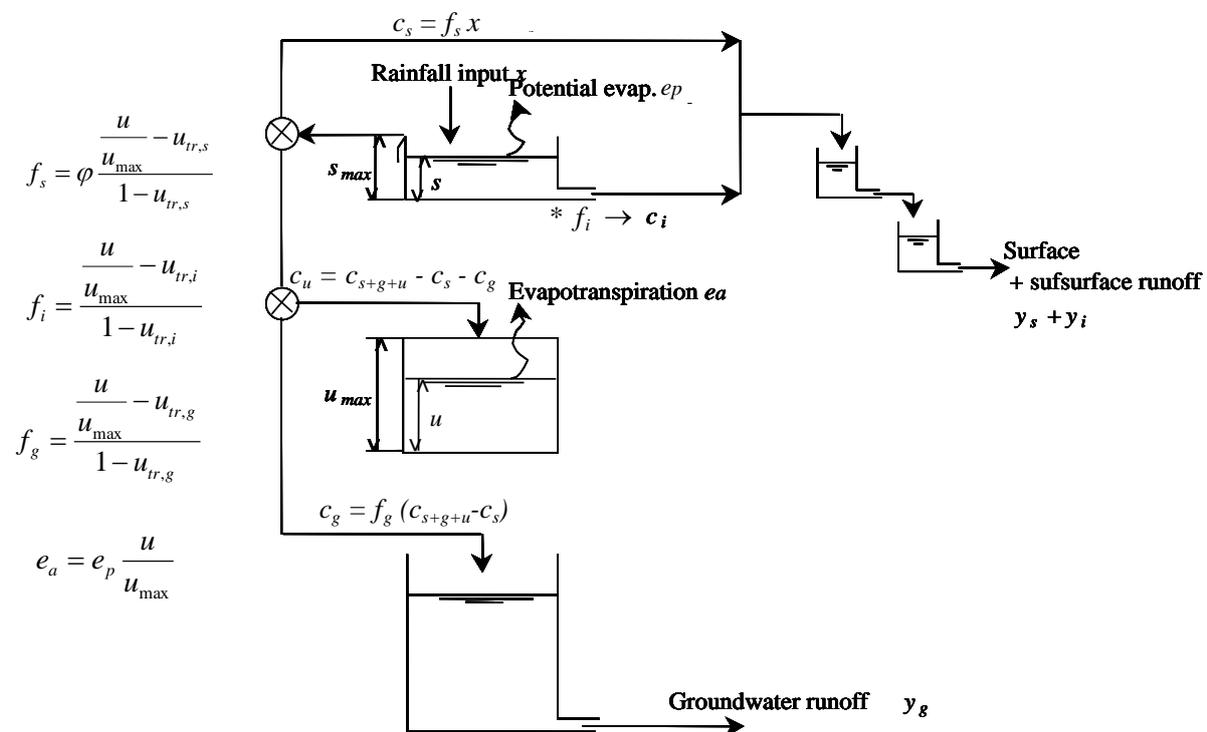
Figure 37. Model-structure of the NAM lumped conceptual rainfall-runoff model.
