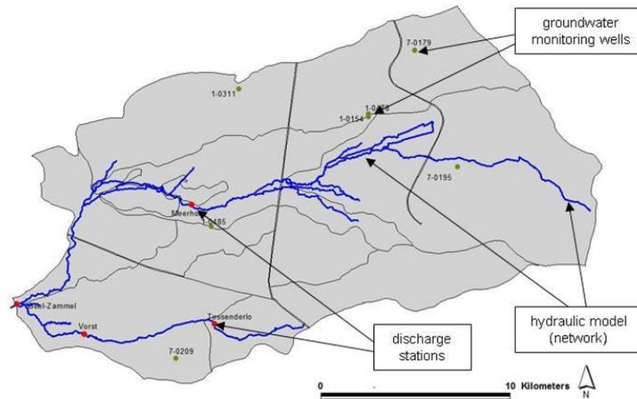
Figure 2. River flow gauging stations location and partial drainage areas for Molsse, Grote Nete and Grote Laak sub-catchments.
