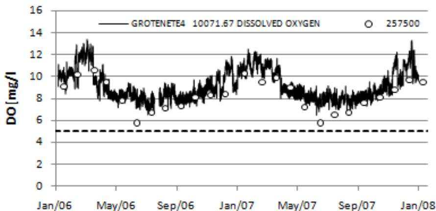
Figure 60. Comparison of observed and modeled DO concentrations at Varendonk station.
