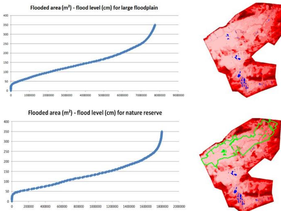
Figure 35: Hypsometric analysis of the Zammelsbroek (top) floodplain and the nature reserve area (bottom)
