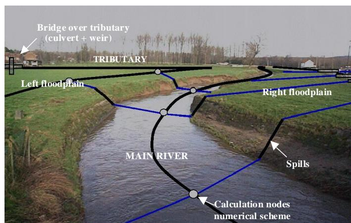
Figure 50. Schematic representation of the quasi-2D approach for river flood modeling (Willems, Vaes et al. 2002).
