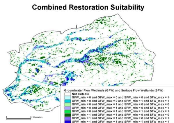
Figure 19: Combined restoration suitability for groundwater dependent wetlands (GFW) and river stage influenced wetlands (SFW).
