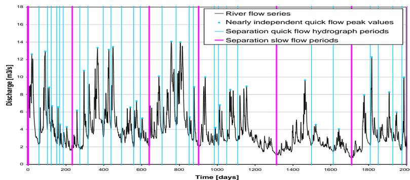
Figure 41 Split of the time series in nearly independent quick and slow flow periods based on the observed series at Varendonk station.
