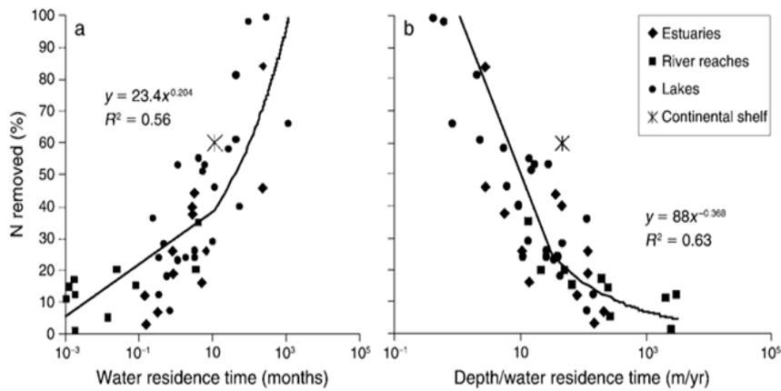
Figure 64: Effect of water residence time on relative N-removal
