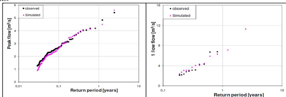
Figure 46. Comparison of observed and simulated (VHM model) peak and low flows vs. return period.
