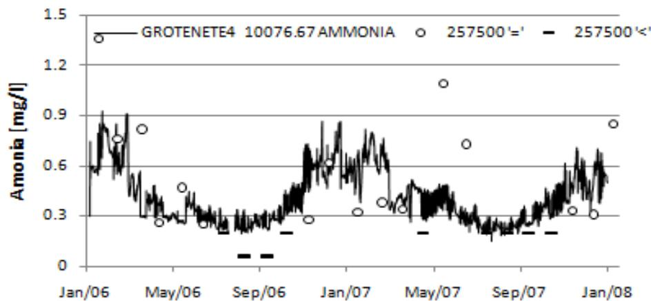
Figure 62. Comparison of observed and modeled NH<sub>4</sub>-N concentrations at Varendonk station.
