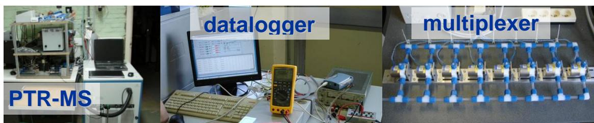
Figure 2: From left to right: (a) PTR-MS set-up, (b) DAQ and (c) multiplexer.
