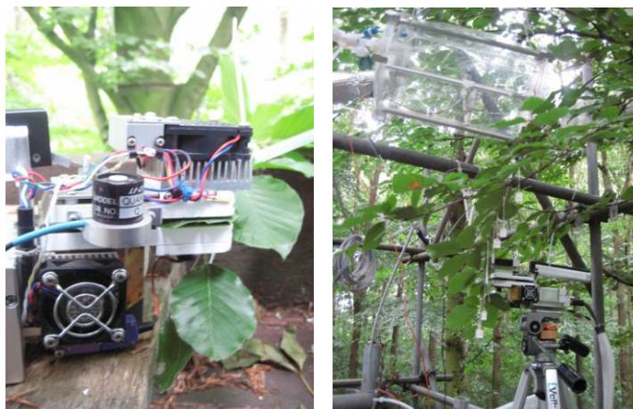
**Figure 26: Portable LI-6400 IRGA in the Aelmoeseneie forest (9 July 2008) to measure offline photosynthesis and transpiration rates**
