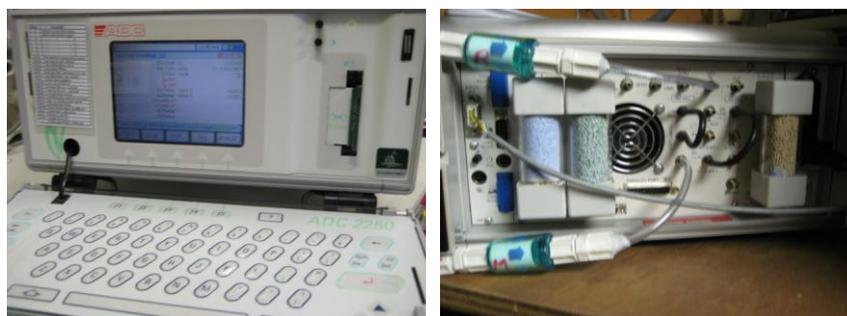
**Figure 23: Stationary ADC 2250 IRGA to measure online photosynthesis and transpiration rates.**
