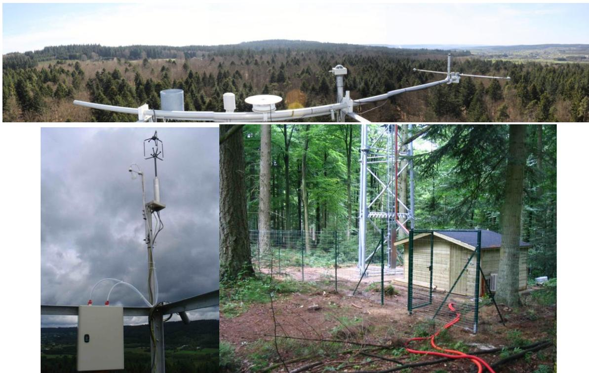
**Figure 33: (a) Panorama at the tower top showing radiation sensors (b) the air sampling inlet close to the sonic anemometer (c) the tower base with the shelter hosting the PTR-MS and acquisition systems.**
