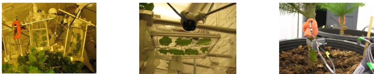
**Figure 1:** (a) View of branches enclosed in the two measuring cuvettes and of the empty reference cuvette, (b) detail of the grid for horizontal and non-overlapping positioning of leaves (c) LVDT (linear variable displacement transducer), TDP (thermal dissipation probe) installation on conifer tree.
