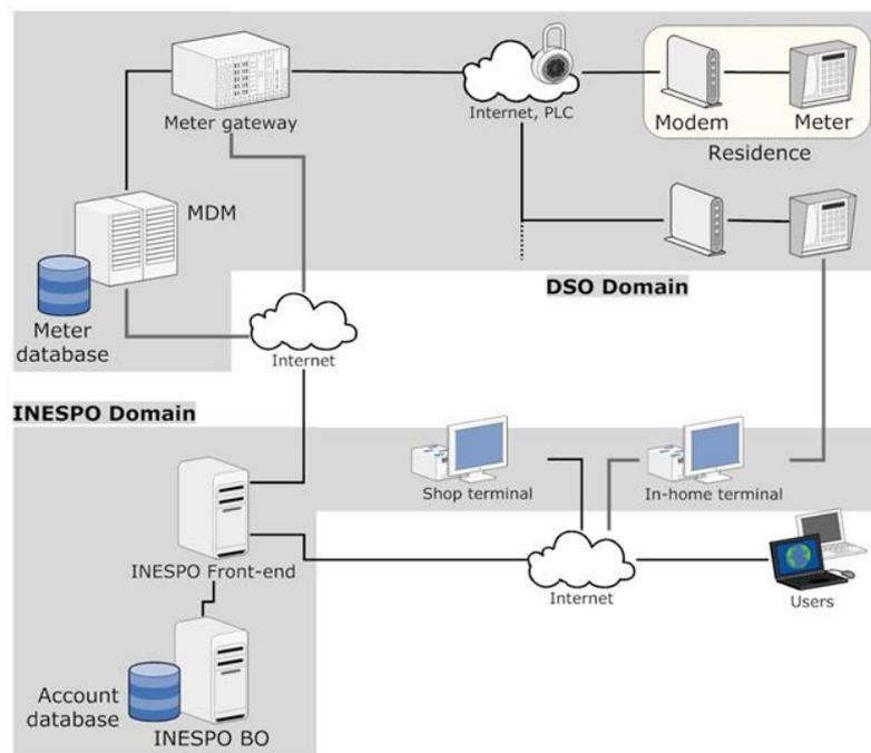
Figure 12 INESPO advanced smart meter architecture outline
