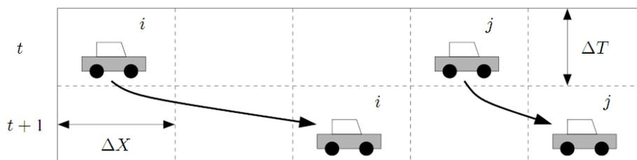
**Figure 1:** Schematic diagram of the operation of a single-lane traffic cellular automaton (TCA); here, the time axis is oriented downwards, the space axis extends to the right. The TCA's configuration is shown for two consecutive time steps  $t$  and  $t+1$ , during which two vehicles  $i$  and  $j$  propagate through the lattice.
