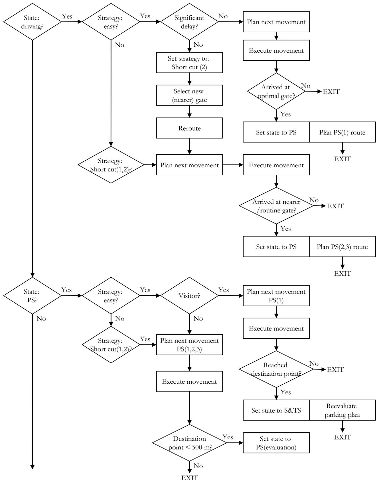
**Figure 17:** Diagram of the behavioural module of the SUSTAPARK model (first part). The arrow at the bottom-left goes to top diamond of figure 19. Further explanations are given in Sections 4.3.1 and 4.3.2.
